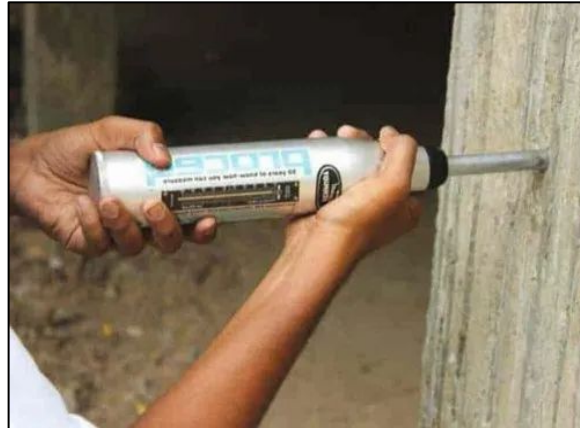
Fig. 1. Rebound hammer test
