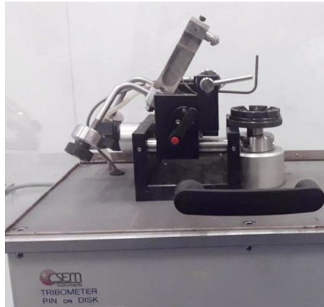
Fig. 3. Pin on disk tribometer
