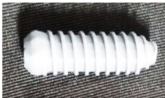
Fig. 3. Interference screw made from PMMA 3D printing product
