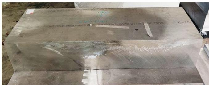
**Fig. 8.** The aluminium 6061-T6 substrate
