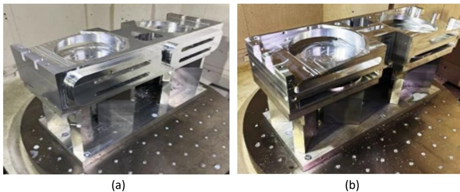
Fig. 21. Fixture of the part during machining (a) OP4 (b) OP2 and OP5
