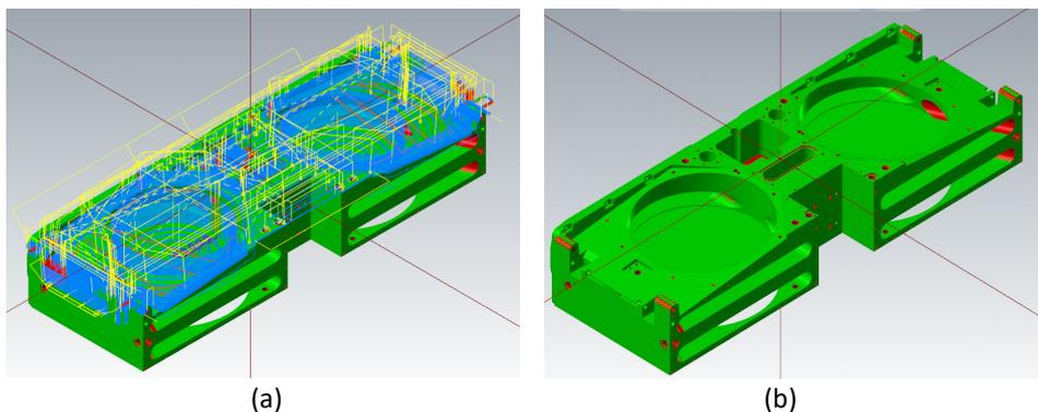
Fig. 16. (a) Tool path overview (b) Stock model for machining OP5
