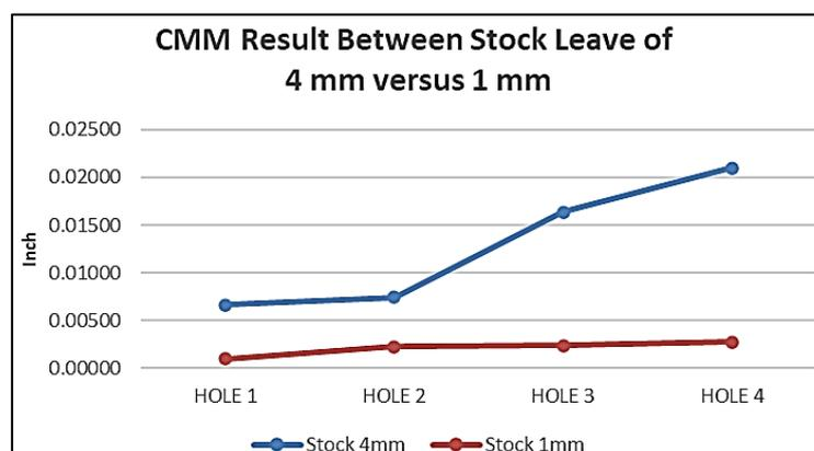
**Fig. 17.** Graph CMM reading of stock leave of 4 mm and 1 mm
