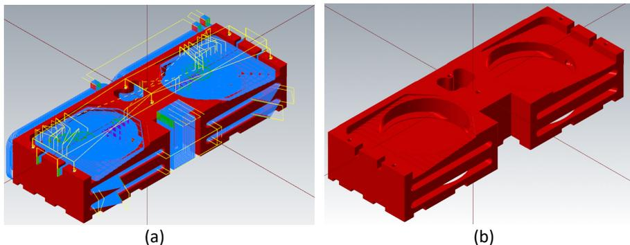
Fig. 12. (a) Tool path overview (b) Stock model for machining OP2
