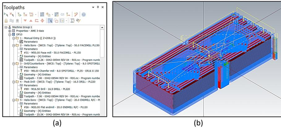
Fig. 3. Tool path manager (a) Tool path overview (b) Displayed graphic
