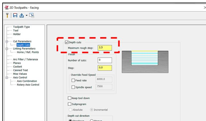
Fig. 7. The depth of cut setting
