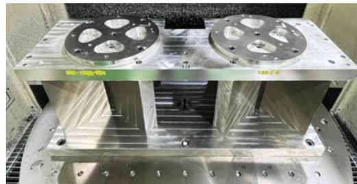
**Fig. 19.** Fixture of the part during machining
