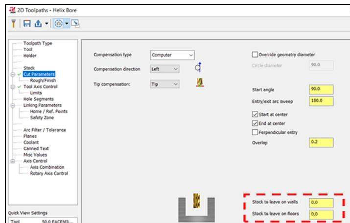
Fig. 6. Setting the stock to leave on walls and the floor
