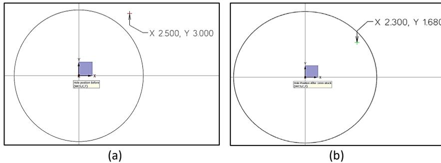
**Fig. 18.** CMM measurement of X and Y coordinate for hole 4 position (a) 4 mm (b) 1 mm
