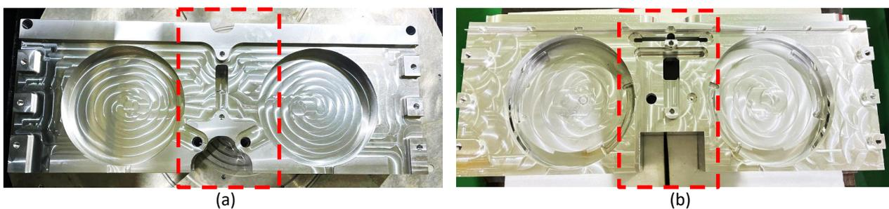
Fig. 22. Actual part finish of machining OP1 with stock leave (a) 4 mm (b) 1 mm
