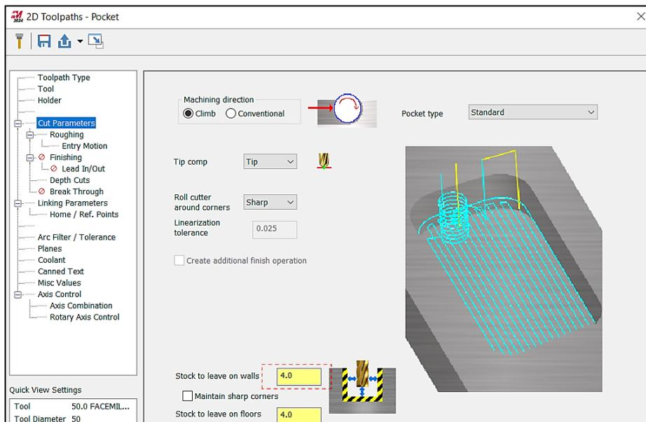
Fig. 13. The stock leave for the floors and walls during machining OP2 is 4mm
