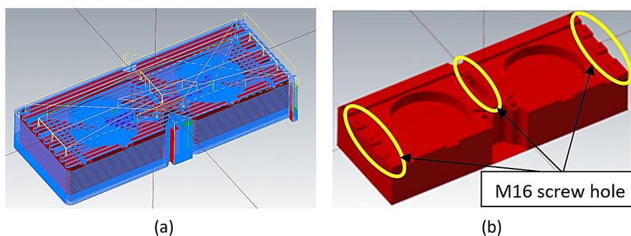
**Fig. 10.** (a) Tool path overview (b) Stock model for machining OP1
