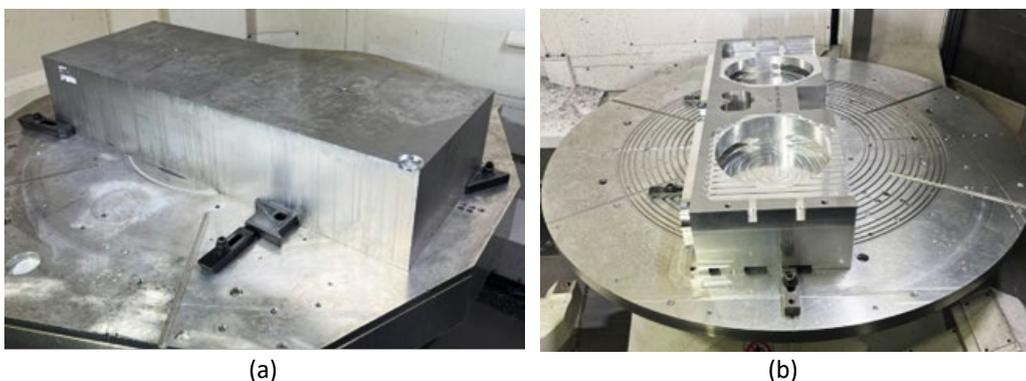
**Fig. 20.** Part setup (a) Machining OP1 (b) Fixture of the part during machining OP3
