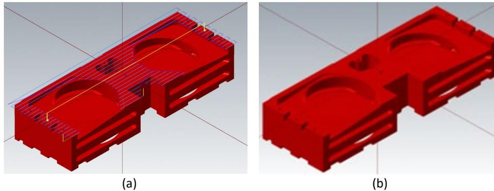
Fig. 14. (a) Tool path overview (b) Stock model for machining OP3
