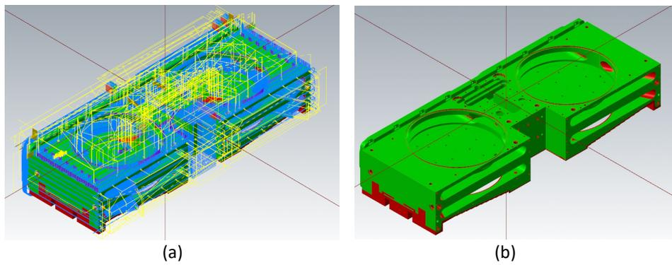
Fig. 15. (a) Tool path overview (b) Stock model for machining OP4
