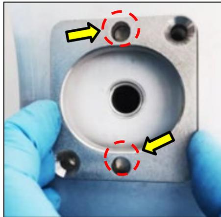
**Fig. 9.** Hole offset due to true position is out of specification
