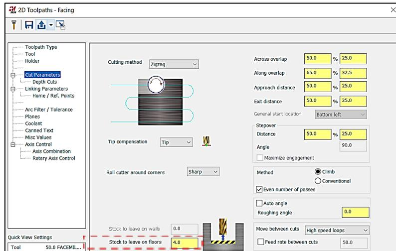
Fig. 11. The stock leave for the floor during machining OP1 is 4 mm
