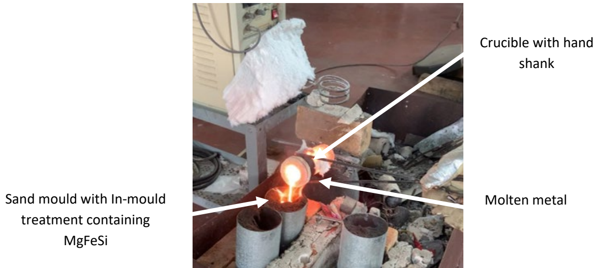
Fig. 1. Experimental setup during melting and alloying
