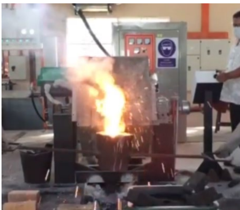
Fig. 1. Experimental setup during molten metal pouring
