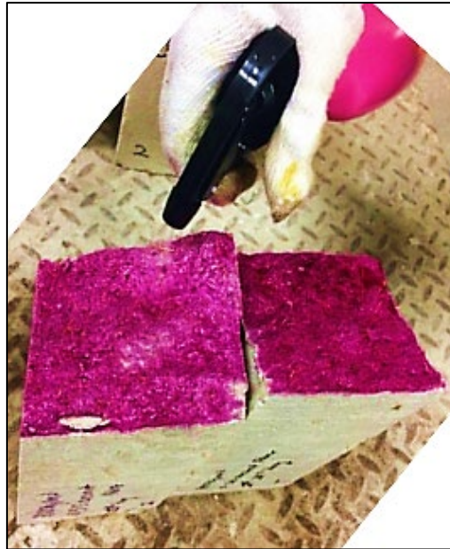
Fig. 2. Phenolphthalein solution was sprayed on the LFC specimen
