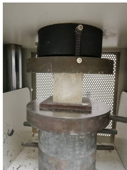
Fig. 4. Apparatus for compression testing
