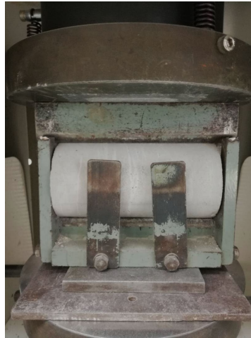
Fig. 5. Setup for splitting tensile test
