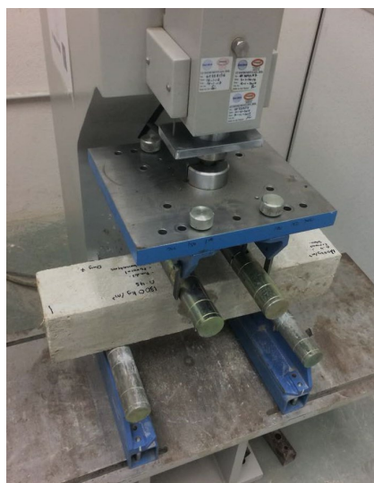
Fig. 6. Setup for three-point flexural test via ELE flexural testing machine
