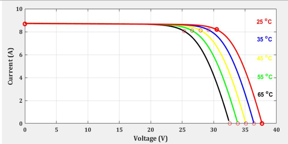
Fig. 7. I-V characteristic at constant solar radiation with different temperature
