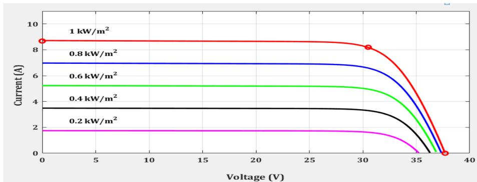
Fig. 5. I-V Characteristics for various conditions of solar Irradiation
