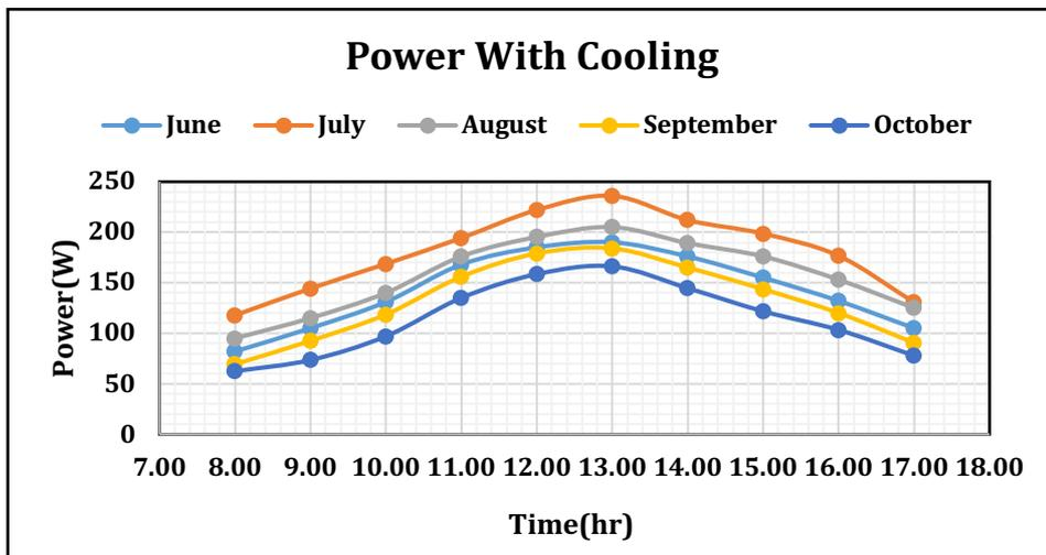
Fig. 10. Electrical Power with cooling at daily time months
