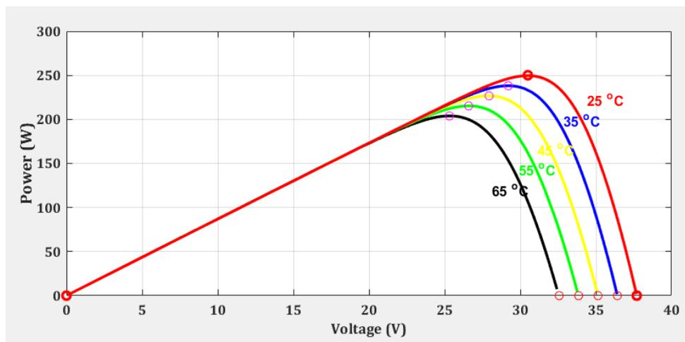
Fig. 8. Effect of temperature on P V characteristics at constant solar radiation
