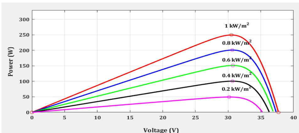
Fig. 6. P-V Characteristics for various conditions of solar Irradiation
