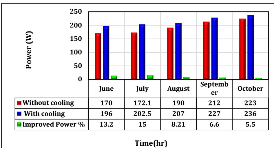
Fig. 13. Improved Power with and without cooling against months
