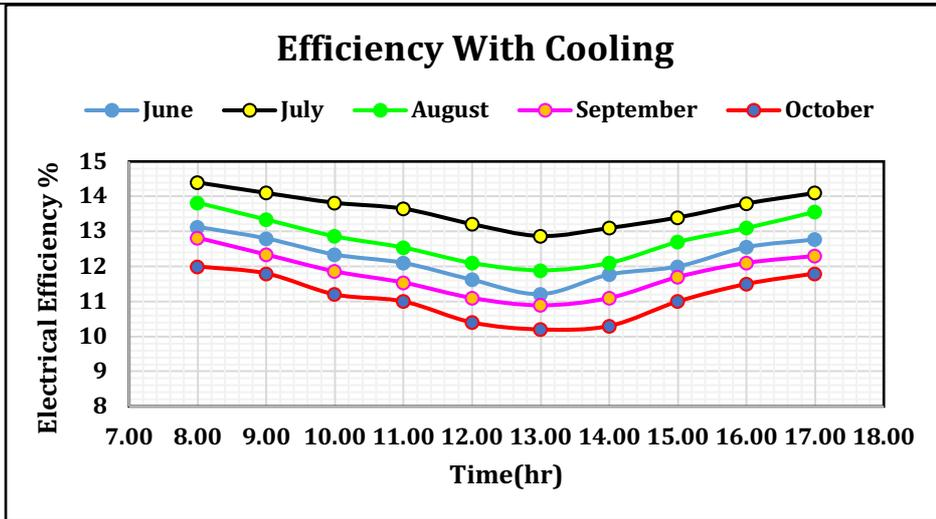
Fig. 11. Efficiency with daily time with cooling system
