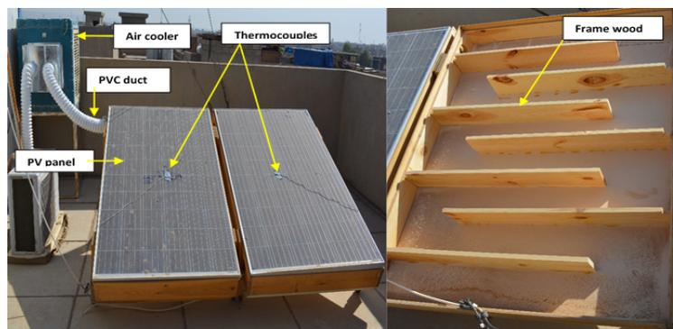
Fig. 4. Experimental device of 250 W Panel
