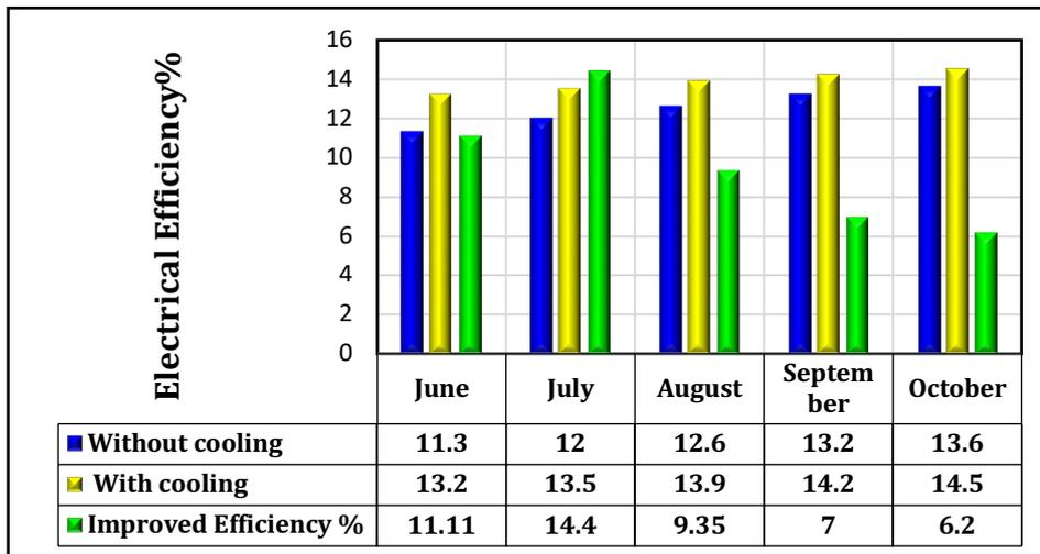
Fig. 14. Improved efficiency with and without cooling against months
