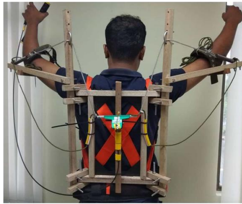
Fig. 2. Developed passive exoskeleton for oil palm harvesting
