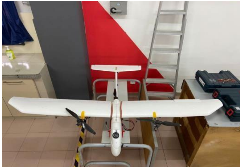
Fig. 2. The hybrid VTOL UAV for research and development in UTHM
