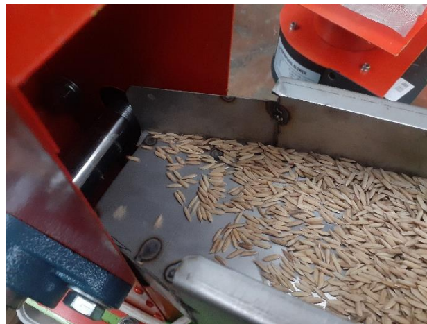
Fig. 9. Vibration feeder of paddy grain cleaner
