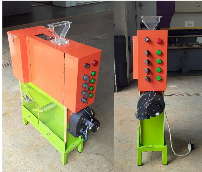
Fig. 7. Developed prototype of paddy grain cleaner
