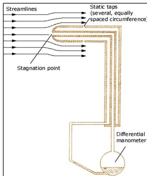
Fig. 4. Working mechanism of pitot tube
