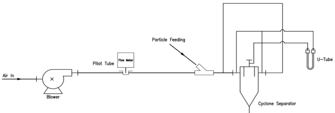
**Fig. 2.** Schematic diagram of dual inlet cyclone separator
