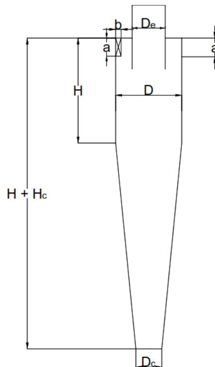
**Fig. 1.** Schematic of cyclone separator structure
