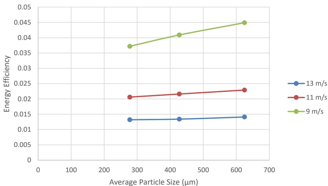
Fig. 5. Effect of average particle size and energy efficiency
