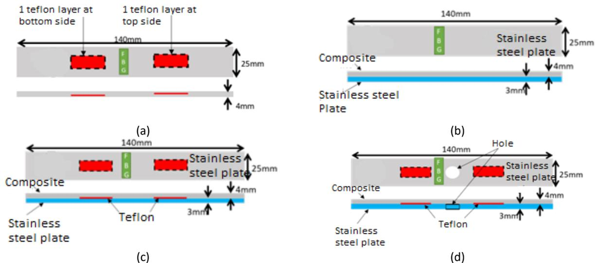
**Fig. 3.** Schematic diagram of composite with FBS sensor location placement (a) Composite with Teflon only (b) stainless steel with patched composite only (c) Stainless steel with patched composite and Teflon (d) holed stainless steel patched with composite and Teflon
