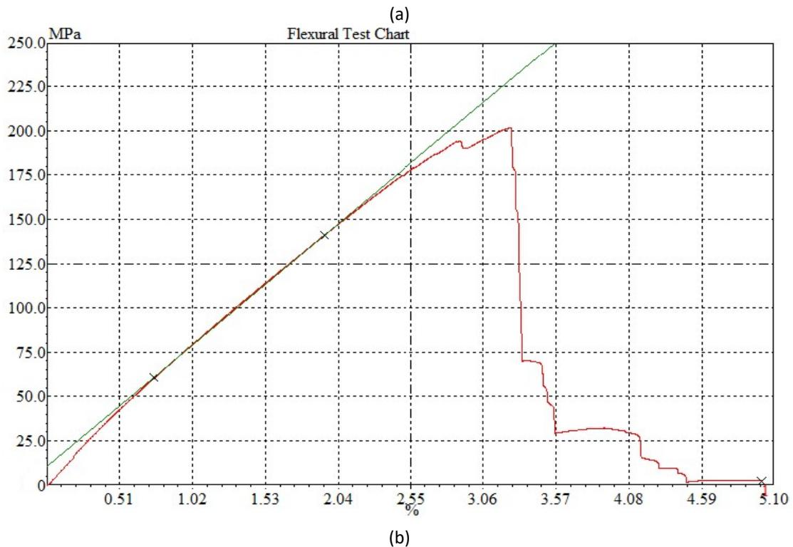
**Fig. 5.** Examples of graph from composite mechanical test (a) FBG sensor response curve (b) UTM machine response curve
