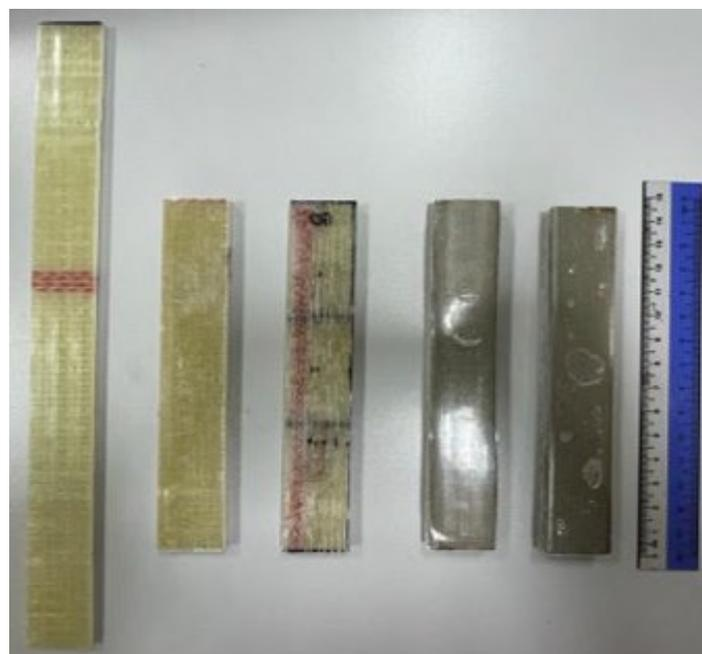
**Fig. 1.** Example of composite samples for mechanical test
