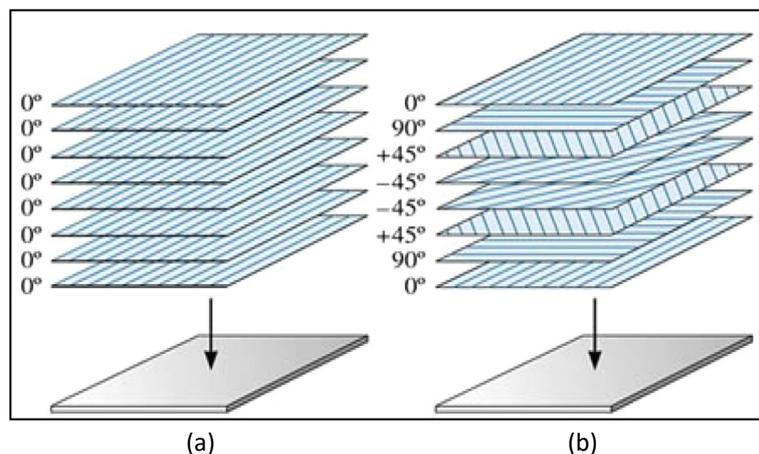
**Fig. 1.** (a) Unidirectional quasi-isotropic (b) cross-piled quasi-isotropic lamination [8]
