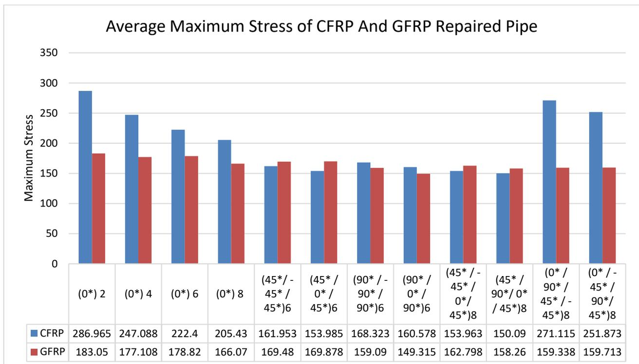
**Fig. 4.** Graph of comparison to compare average maximum stress in between CFRP and GFRP
