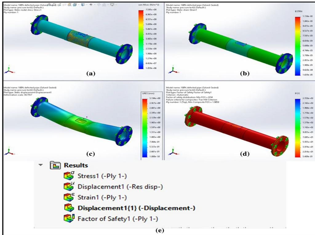
**Fig. 3.** (a) The sample stress results (b) the sample strain results (c) the sample displacement results (d) the sample factor of safety results (e) the list of results that could be achieved by static analysis
