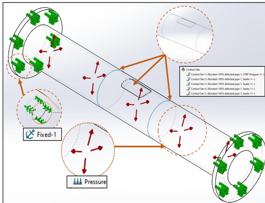
**Fig. 2.** The assembled components were then defined with fixed geometry, contact set and internal pressure for static analysis
