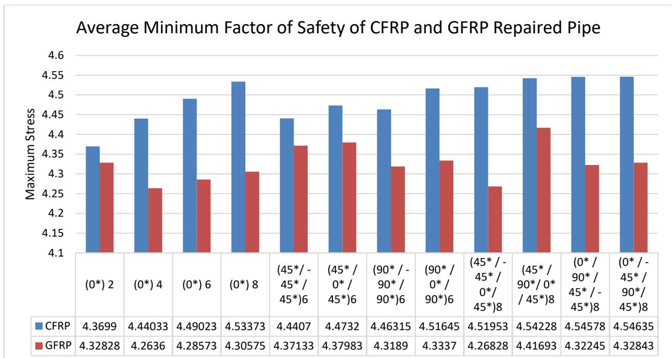
**Fig. 5.** Graph of comparison to compare average minimum factor of safety between CFRP and GFRP repaired pipe
