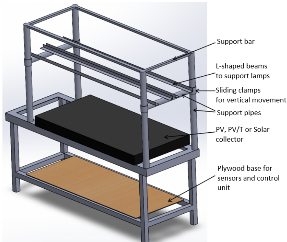
Fig. 1. Isometric View of the Solar Simulator Frame
