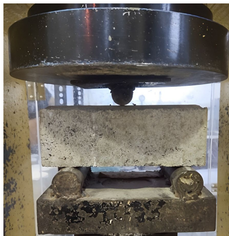
Fig. 5. Flexural strength test setup
