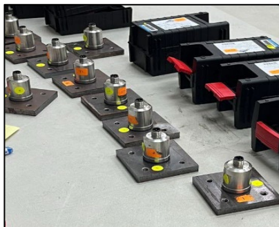
Fig. 2. Accelerometers on steel plate
