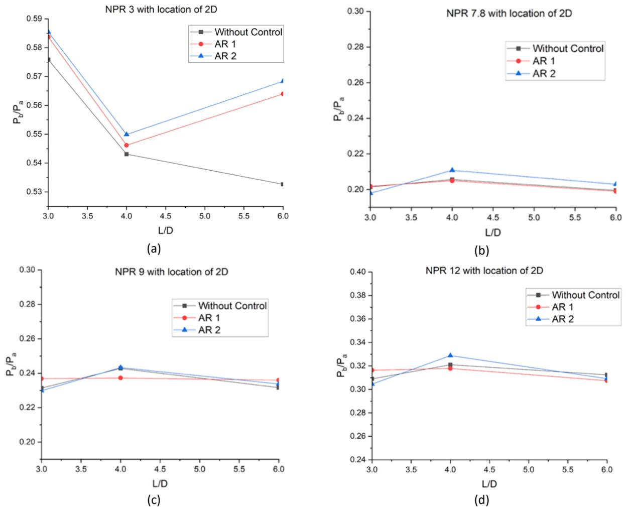
**Fig. 5.** Base pressure ratio varies with  $L/D$  at various locations at 2D
