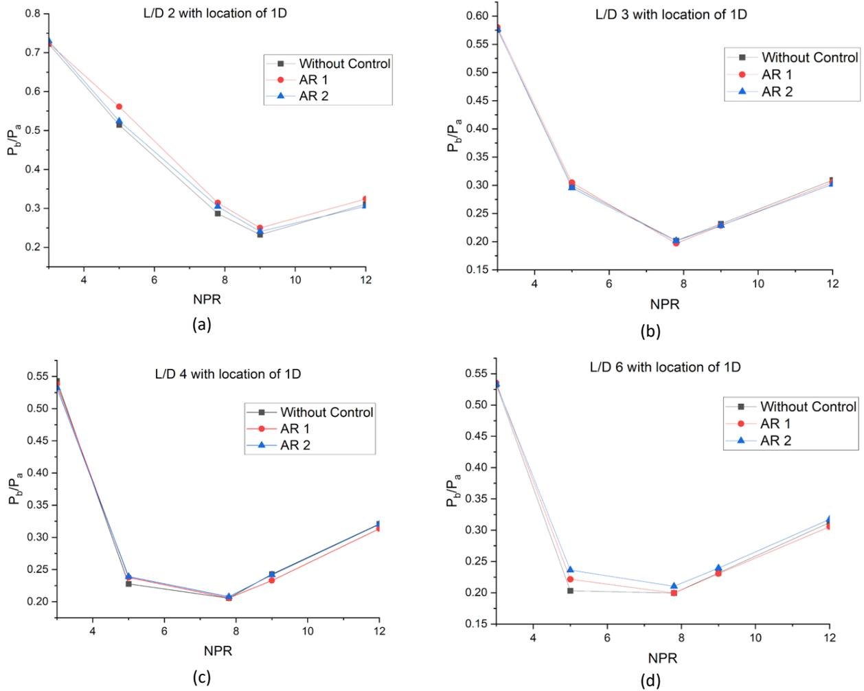
**Fig. 8.** Base pressure ratio varies with NPR for cavity location at 1D
