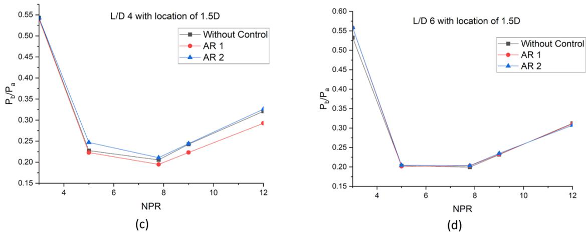
Fig. 9. Base pressure ratio varies with NPR at 1.5D cavity locations.
