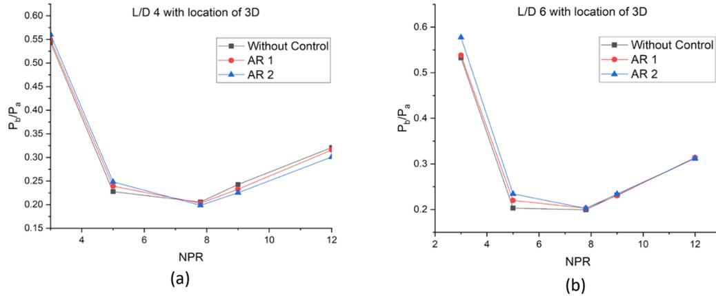
Fig. 11. Base pressure ratio varies with NPR for a cavity location 3D
