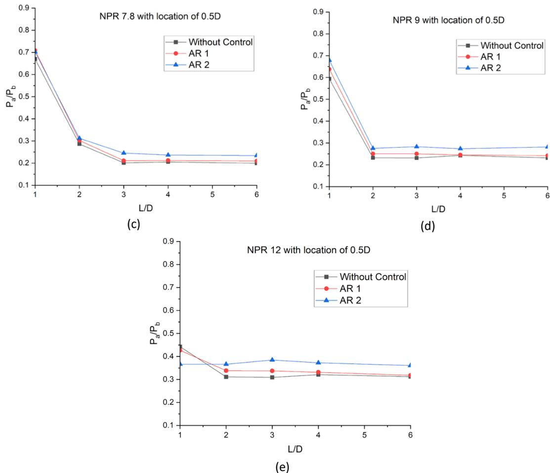
**Fig. 2.** Base pressure ratio variations with  $L/D$  at numerous locations of 0.5D
