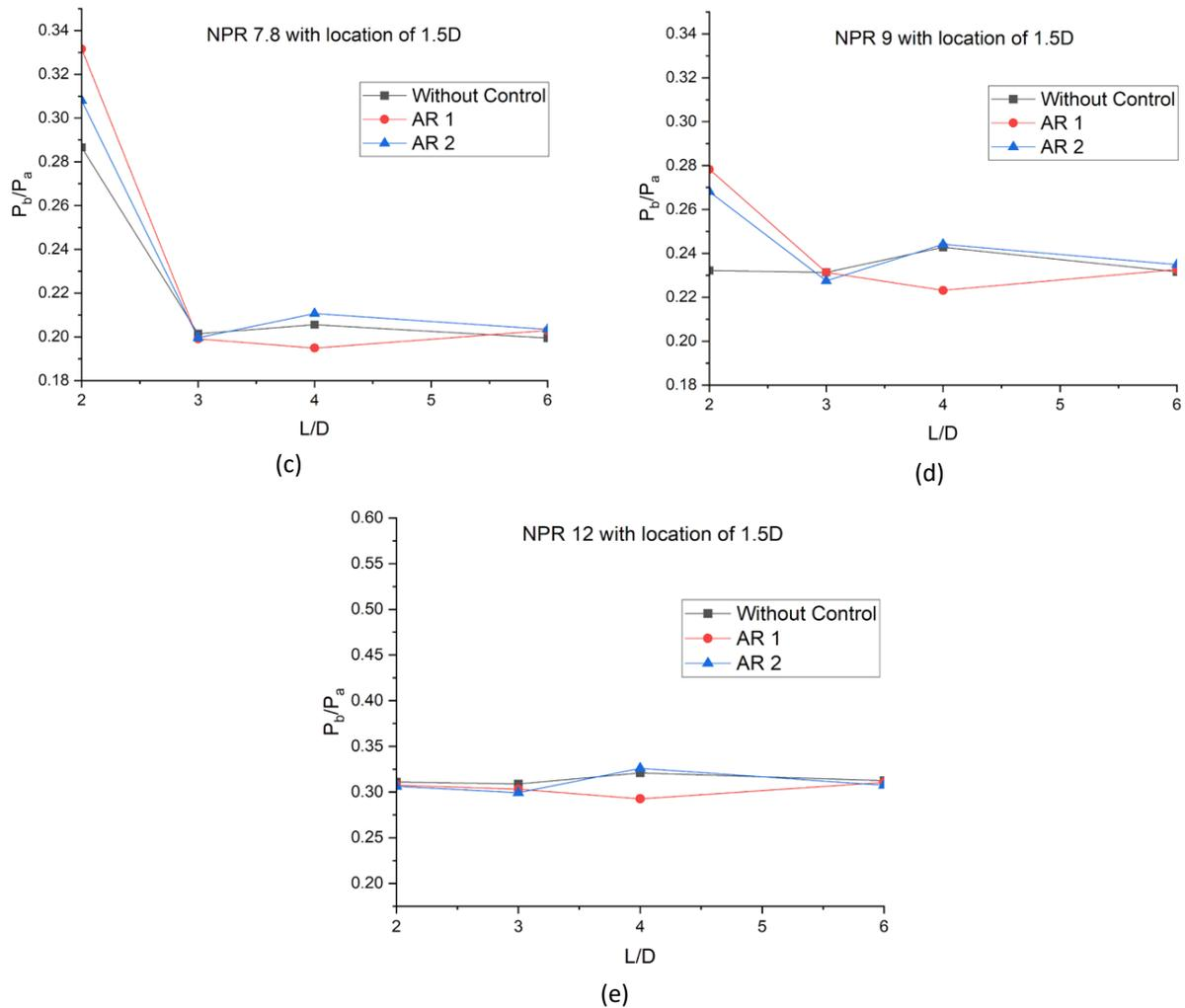
**Fig. 4.** Base pressure variation with  $L/D$  for both plain duct and duct with control
