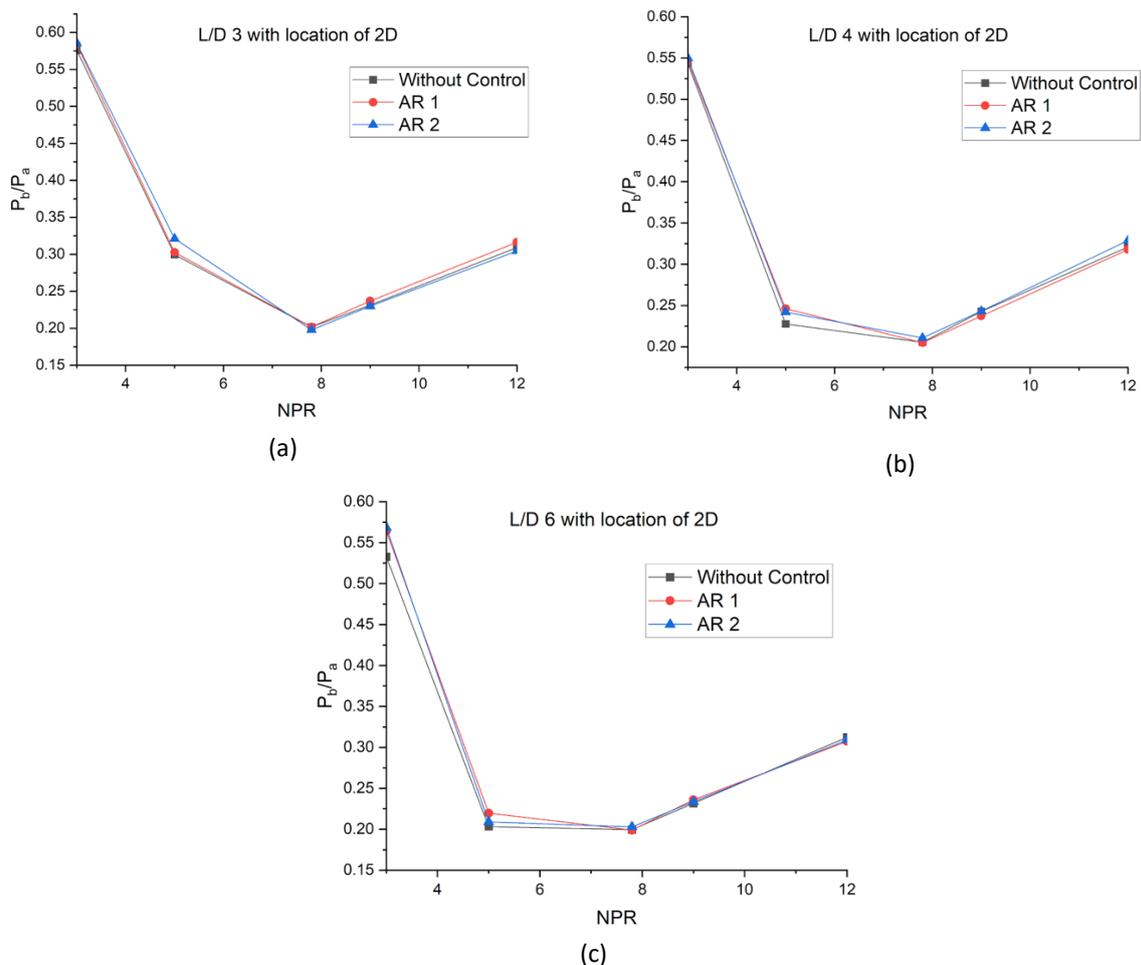
Fig. 10. Base pressure ratio varies with NPR for cavities located at 2D
