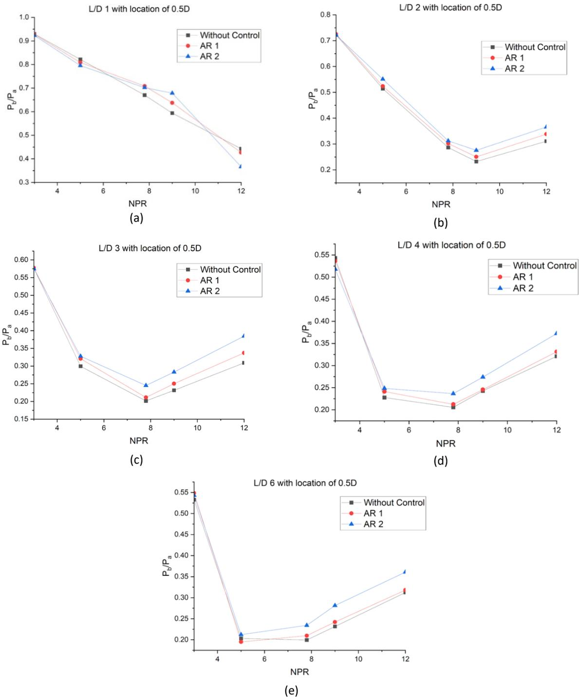
**Fig. 7.** Base pressure ratio variation with NPR for cavity location at 0.5D
