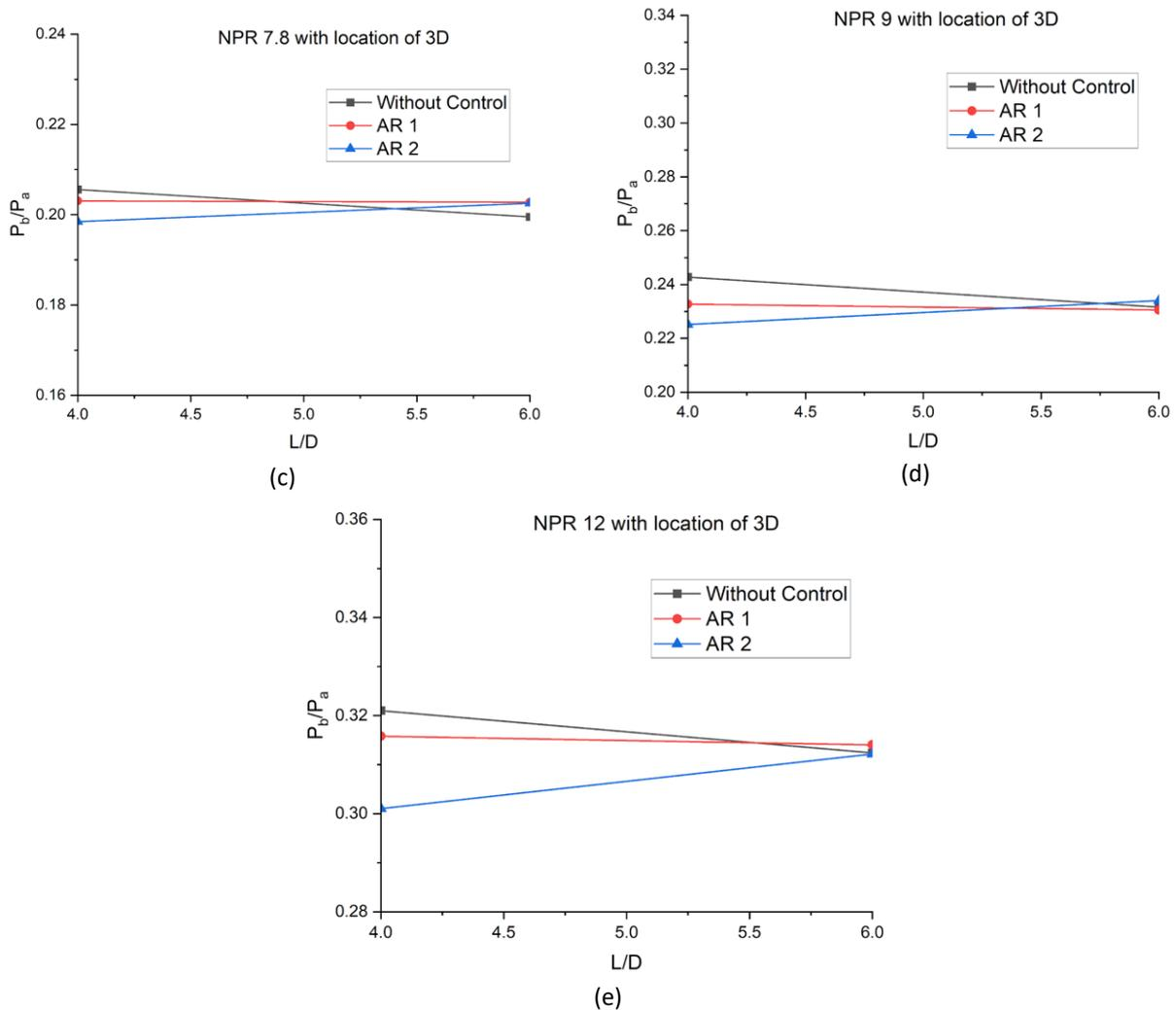
**Fig. 6.** At different locations of 3D, the ratio of the base pressure to the total pressure varies for both plain duct and duct with control with  $L/D$
