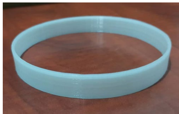
Fig. 2. Samples holder made from ABS
