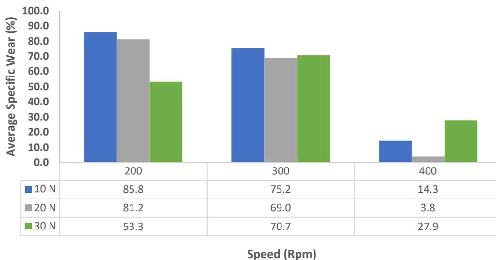
**Fig. 12.** Percentage (%) of difference on the average specific wear rates between the unforged dry sliding and wet sliding cases of Aluminium ER 5356 at different speeds (rpm) and loads (N)
