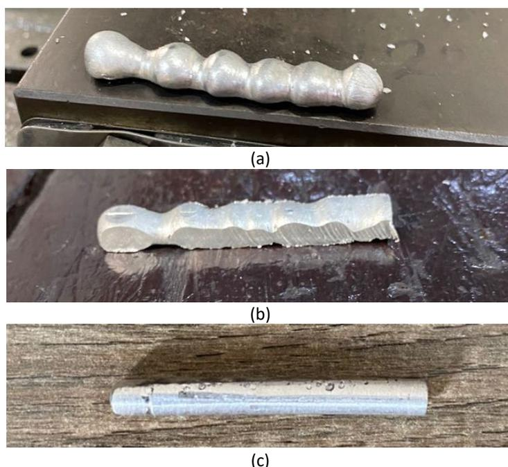
**Fig. 4.** The specimen preparation steps (a) as deposited (b) post-deformation and (c) after machined specimen
