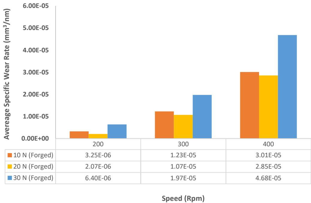
**Fig. 9.** Average specific wear rates of Aluminium ER 5356 on the forged wet sliding cases at different speeds (RPM) and loads (N)
