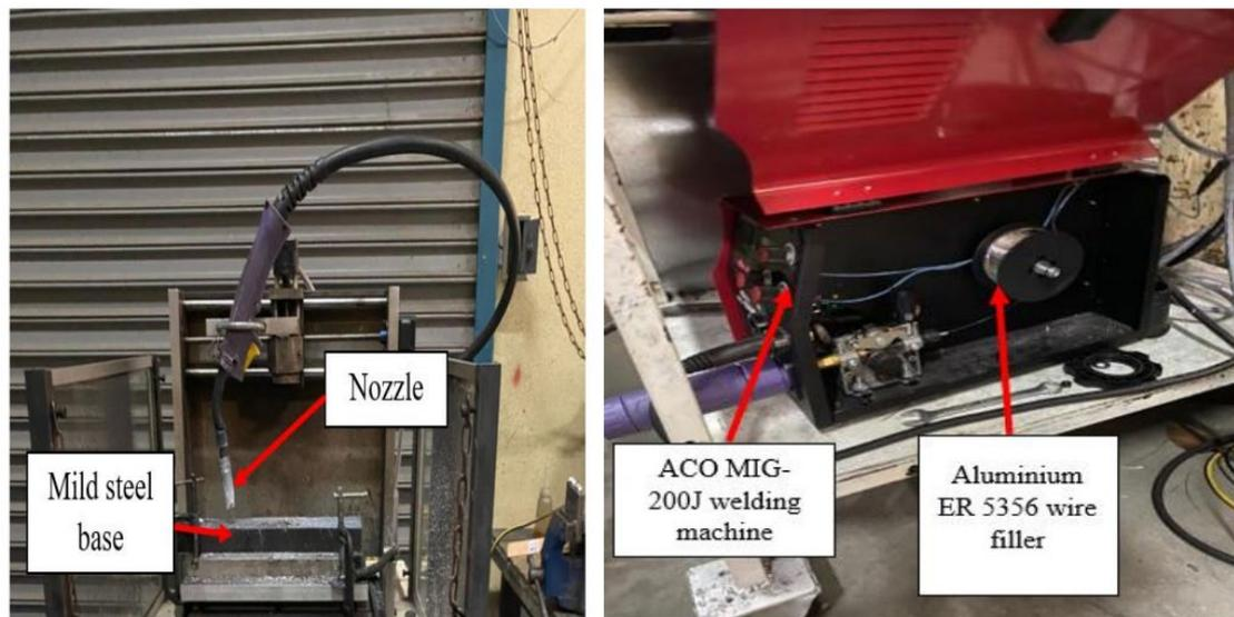
Fig. 1. MiG based 3D welding machine setup
