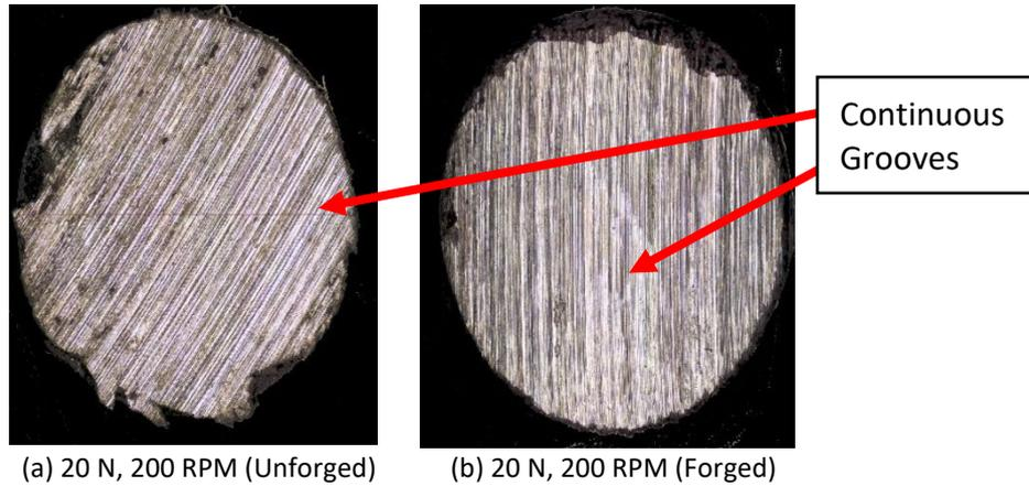
(a) 20 N, 200 RPM (Unforged) (b) 20 N, 200 RPM (Forged)
