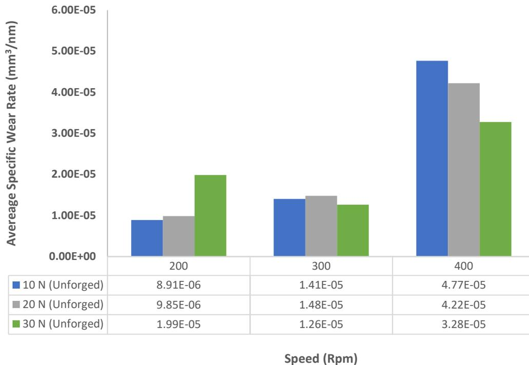
**Fig. 8.** Average specific wear rates of Aluminium ER 5356 on the unforaged wet sliding cases at different speeds (RPM) and loads (N)
