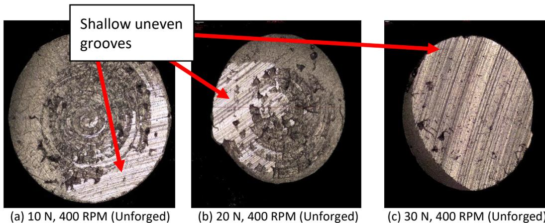
(a) 10 N, 400 RPM (Unforged) (b) 20 N, 400 RPM (Unforged) (c) 30 N, 400 RPM (Unforged)
