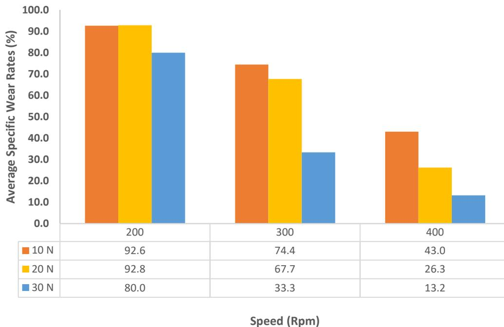
**Fig. 13.** Percentage (%) of difference in the average specific of wear rates between the forged dry sliding and wet sliding cases of Aluminium ER 5356 at different speeds (rpm) and loads (N)
