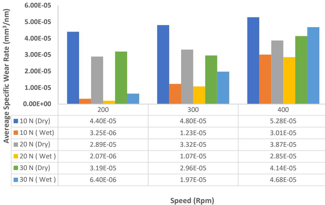
**Fig. 11.** Average specific wear rates of Aluminium ER 5356 on the forged dry and wet sliding cases at different speeds (rpm) and loads (N)
