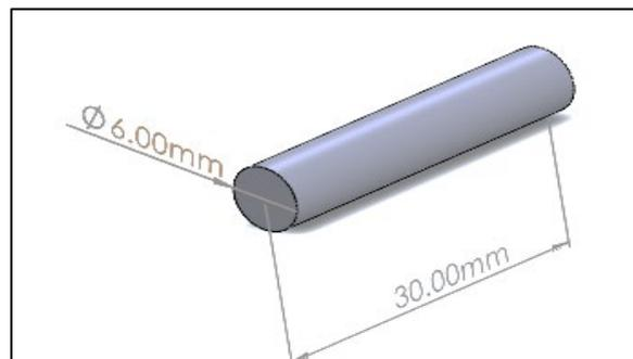
**Fig. 3.** Dimension of the cylindrical flat end pin (unit in mm)
