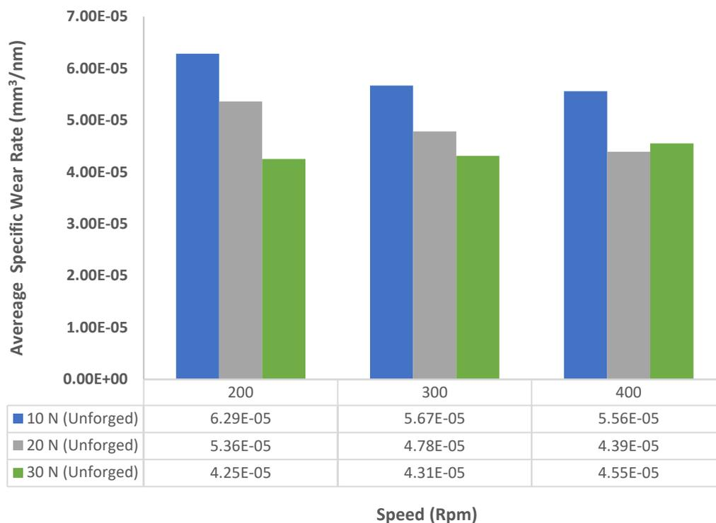
**Fig. 6.** Average specific wear rates of Aluminium ER 5356 on the unforged dry sliding cases at different speeds (RPM) and loads (N)
