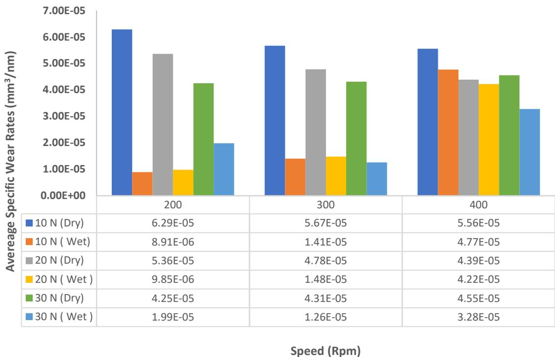
**Fig. 10.** Average specific wear rates of Aluminium ER 5356 on the unforged dry and wet sliding cases at different speeds (rpm) and loads (N)
