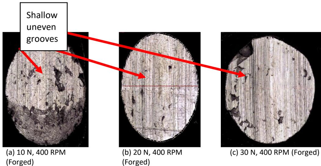
**Fig. 18.** Abrasive wear found in the forged wet sliding cases at 400 RPM and different loads
