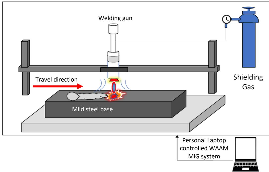
**Fig. 2.** Schematic diagram of the 3D welding machine
