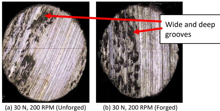
(a) 30 N, 200 RPM (Unforged) (b) 30 N, 200 RPM (Forged)
