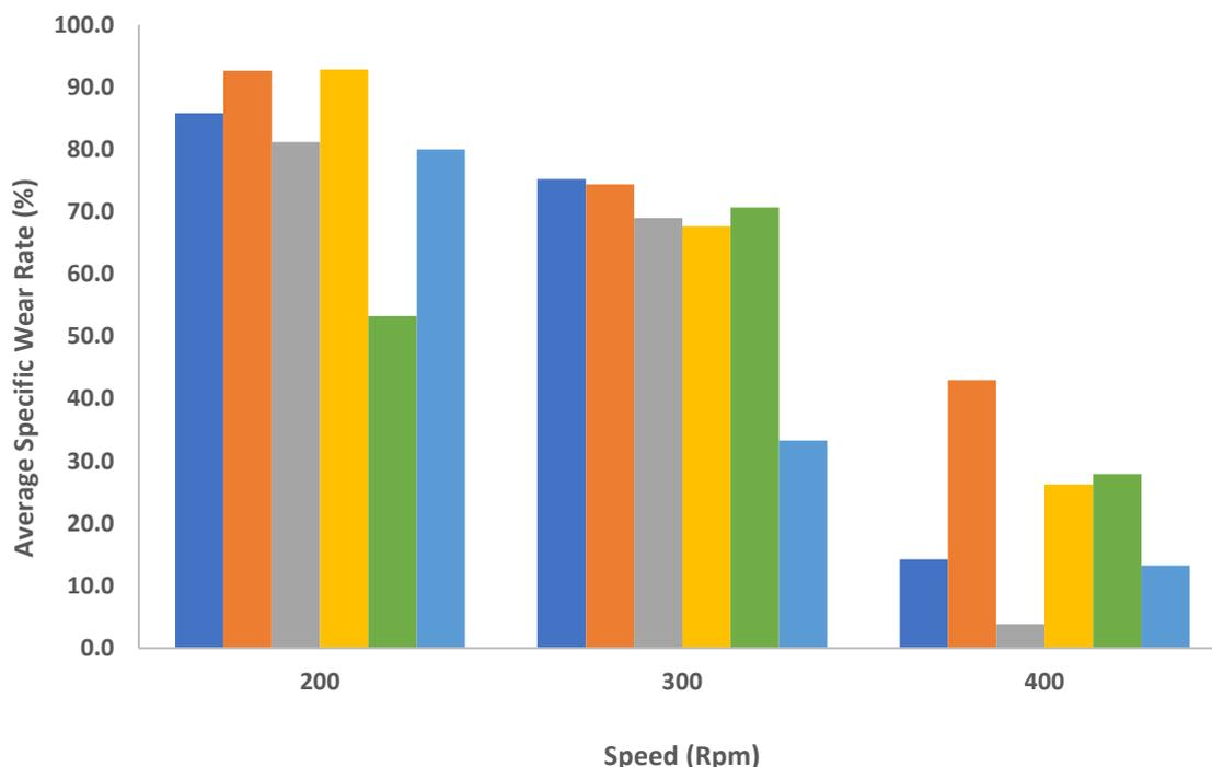
**Fig. 14.** Percentage (%) of difference in the average specific of wear rates between the unforged and forged dry and wet sliding cases of Aluminium ER 5356 at different speeds (RPM) and loads (N)
