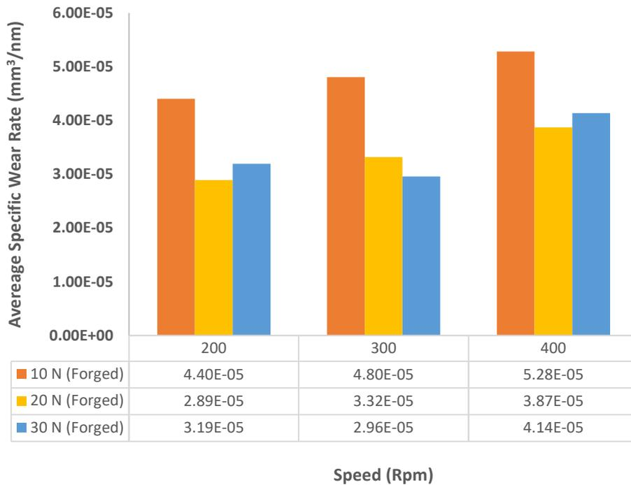
**Fig. 7.** Average specific wear rates of Aluminium ER 5356 on the forged dry sliding cases at different speeds (RPM) and loads (N)
