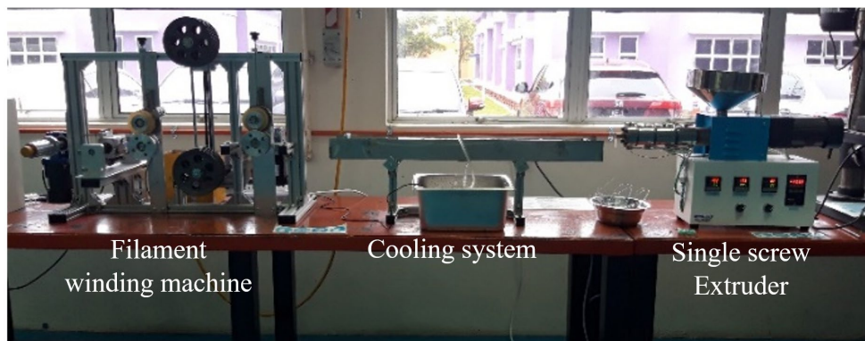
Fig. 2. 3D Printing filament fabrication process
