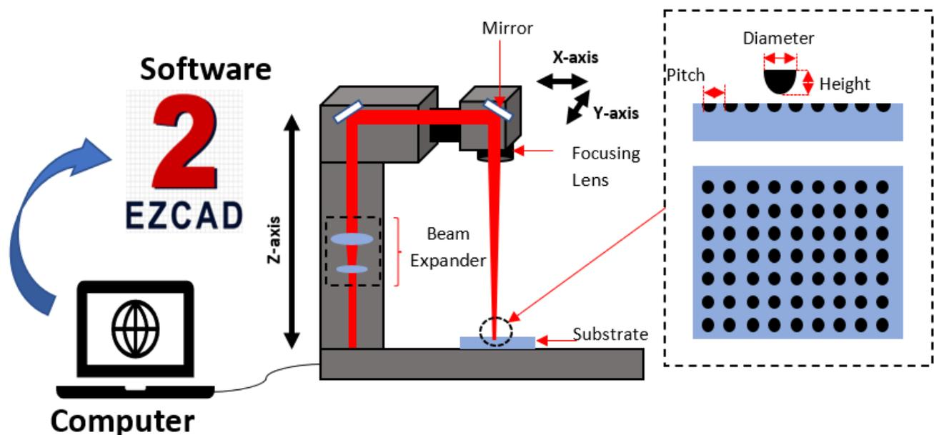
Fig. 1. Schematic diagram for the patterning of micro-dots using direct CO<sub>2</sub> laser structuring
