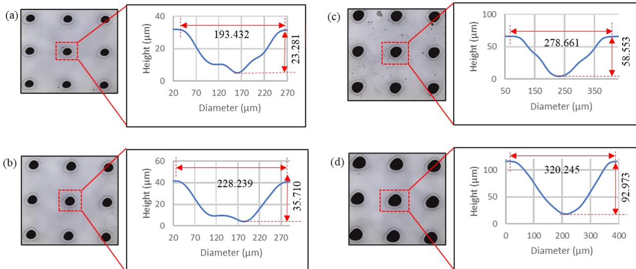
**Fig. 3.** LSCM top view image of the direct laser structured micro-dots (left) and its corresponding LSCM cross section profile (right) at different laser power and constant scanning speed of  $1500 \text{ mmsec}^{-1}$  (a) 2 W (b) 4 W (c) 6 W and (d) at laser power 8 W
