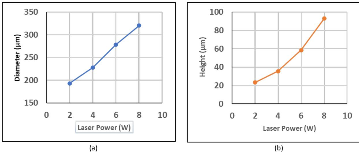
**Fig. 6.** Effect of different laser power at constant scanning speed  $1500 \text{ mmsec}^{-1}$  to the formation micro-dots (a) diameter and (b) height respectively
