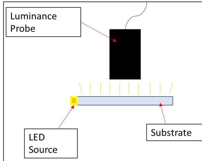
**Fig. 2.** Schematic diagram for the measurement of the luminance reading using SM208 luminance meter
