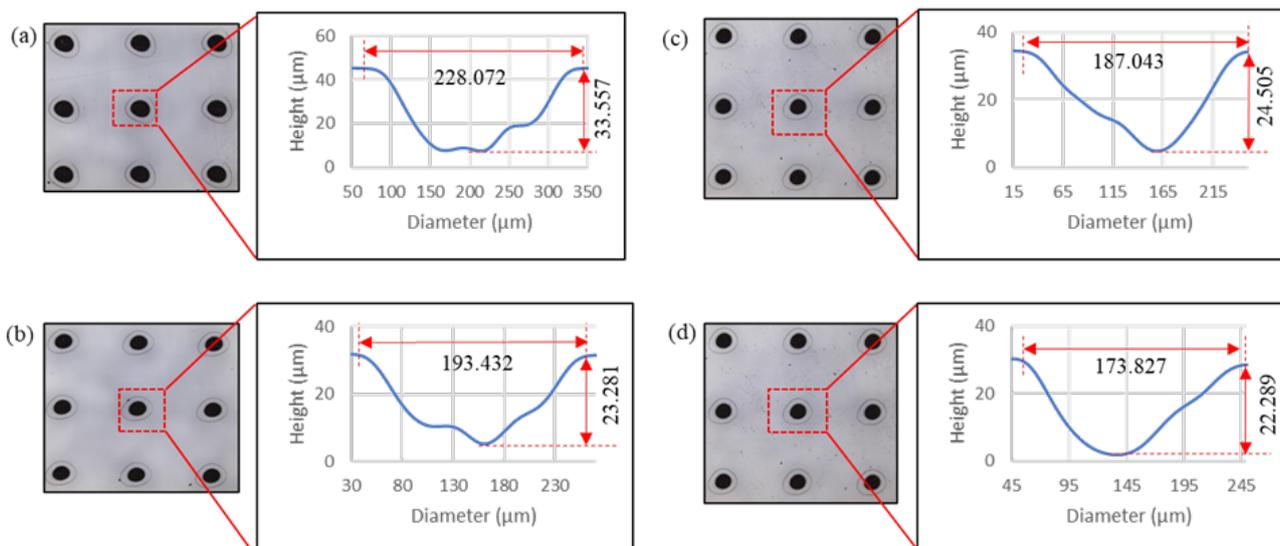
**Fig. 7.** LSCM top view image of the direct laser structured micro-dots (left) and its corresponding LSCM cross section profile (right) at different laser scanning speed and constant power of  $2 \text{ W}$  (a)  $1000 \text{ mmsec}^{-1}$  (b)  $1500 \text{ mmsec}^{-1}$  (c)  $2000 \text{ mmsec}^{-1}$  and (d) at laser scanning speed  $2500 \text{ mmsec}^{-1}$
