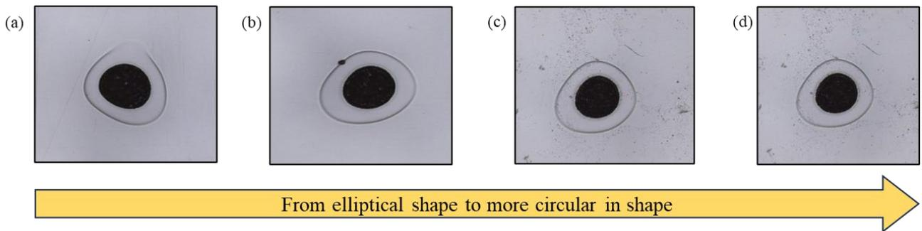
**Fig. 8.** The enlargement of LSCM top view image of the micro-dots from laser scanning speed of (a) 1000  $\text{mmsec}^{-1}$ , (b) 1500  $\text{mmsec}^{-1}$ , (c) 2000  $\text{mmsec}^{-1}$  and (d) 3000  $\text{mmsec}^{-1}$  (right). This photo image shows that the shape of the micro-dots become more circular in shape with the increasing of laser scanning speed
