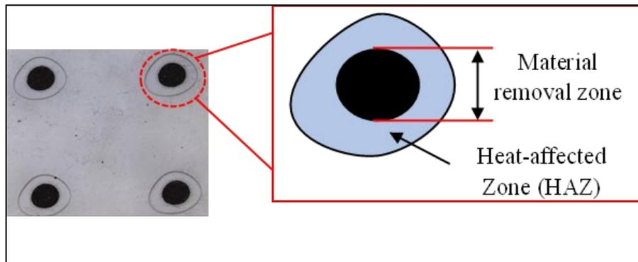
**Fig. 5.** LSCM image (left) and the illustration (right) of the presence of the heat-affected zone (HAZ) along the outer rings of the micro-dots
