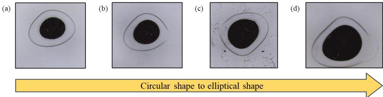
**Fig. 4.** The enlargement of LSCM top view image of the micro-dots from laser power of (a) 2 W (left), (b) 4 W, (c) 6 W to the highest laser power of (d) 8 W (right). These photo images show that the shape of the micro-dots evolved from circular shape to elliptical shape as the laser power increases
