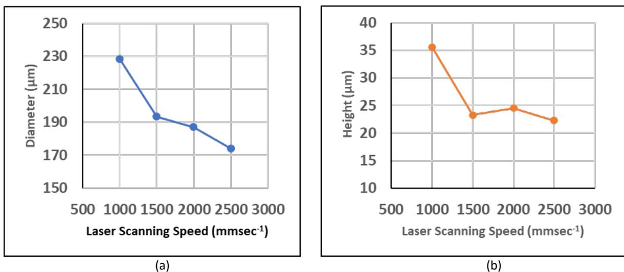
**Fig. 9.** (a) Effect of different laser scanning speed to the formation micro-dots diameter and (b) effect of different laser scanning speed to the formation of micro-dots height
