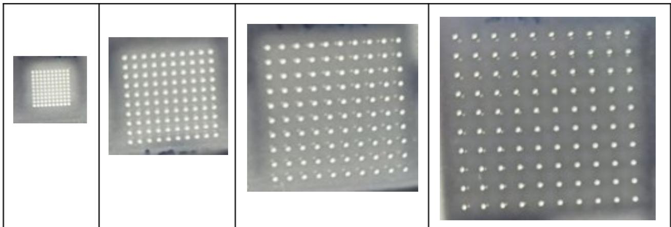
**Fig. 10.** Different brightness from different pitch of micro-dots
