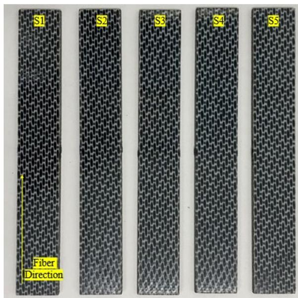
Fig. 3. Set of Tensile Test Specimens
