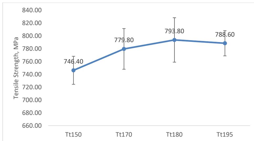
**Fig. 8.** Tensile Strength of CF/PPS Composites Subjected to Different Tool Temperature
