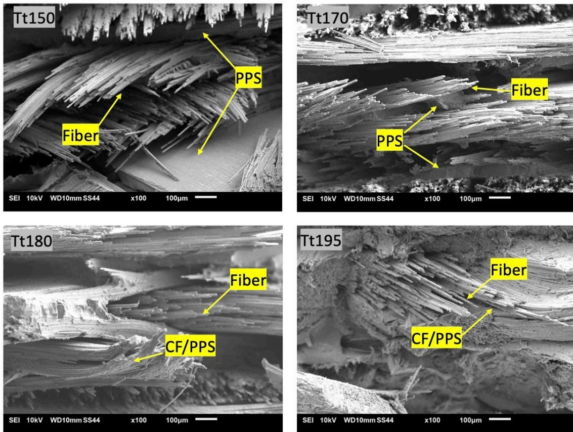
Fig. 9. Failure Mode of Tensile Specimens under SEM
