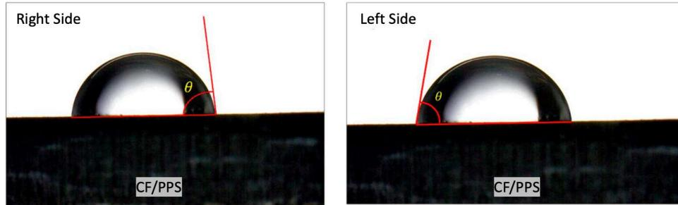
**Fig. 2.** Contact Angle of Water droplet at Right Side and Left Side
