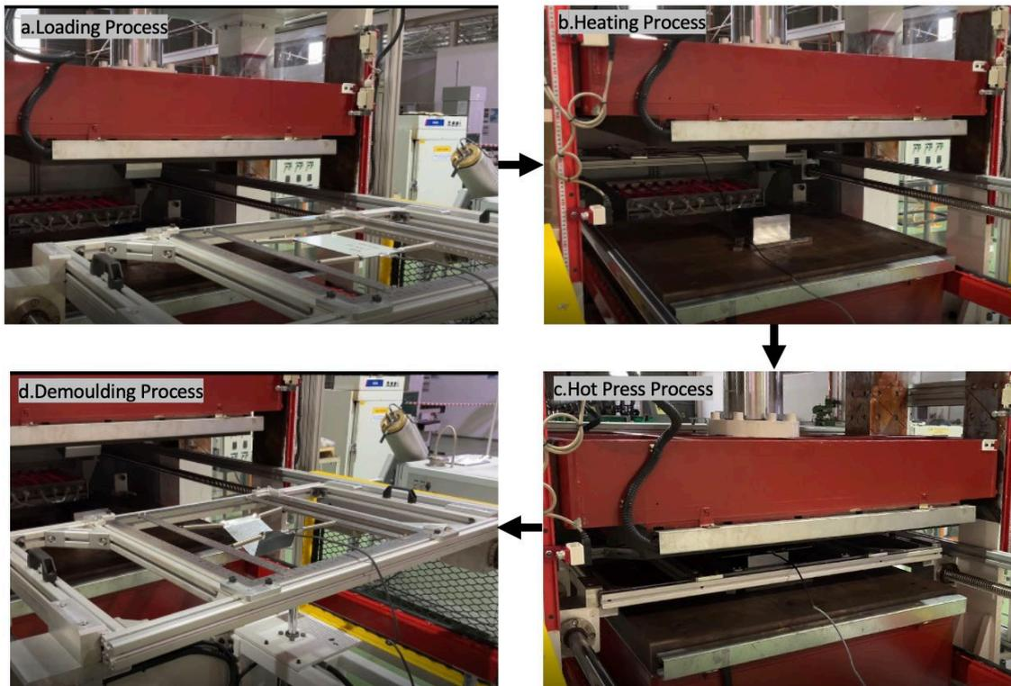
**Fig. 1.** Overview of Hot Press Forming Process
