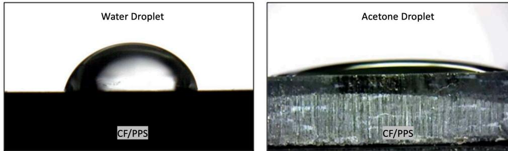
Fig. 4. Water and Acetone Droplets on the CF/PPS Composite Component
