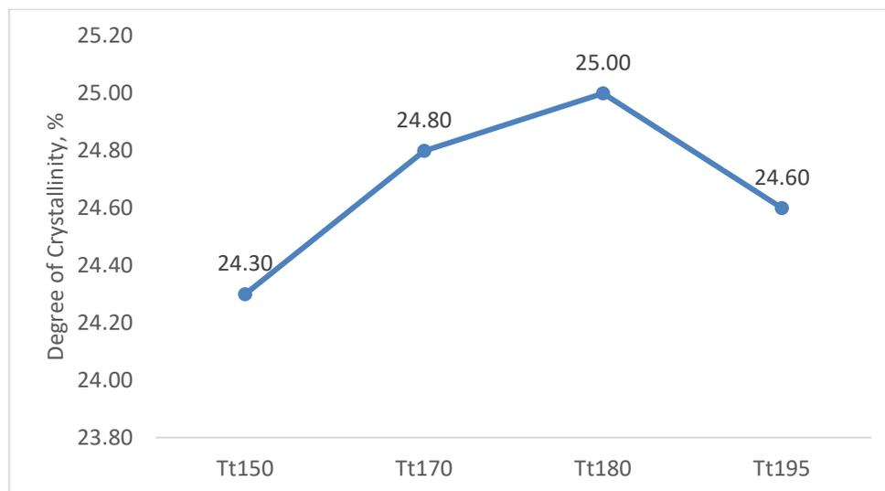
**Fig. 6.** DoC of CF/PPS Composites Subjected to Different Tool Temperature
