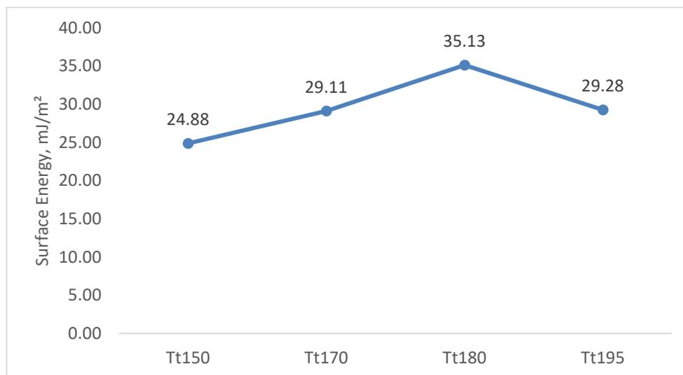
Fig. 5. SE of CF/PPS Composite subjected to Different Tool Temperature
