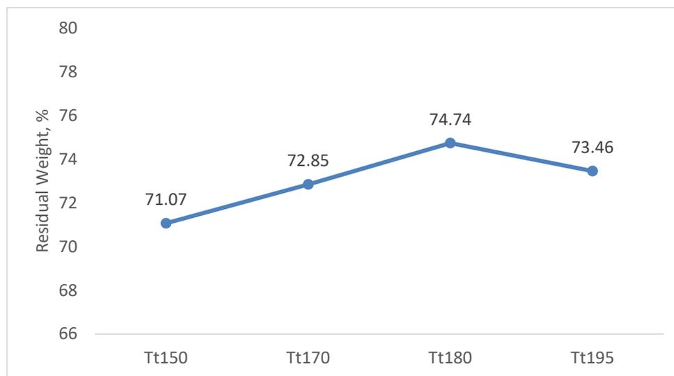
**Fig. 7.** TGA of CF/PPS Composites Subjected to Different Tool Temperature
