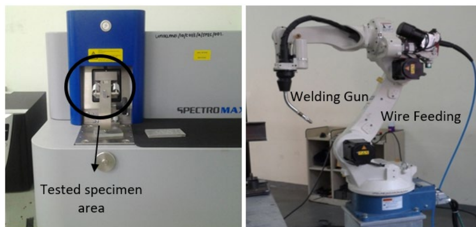
Fig. 2. Material Composition Tested Machine (left) and Arc Welding Robot (right)
