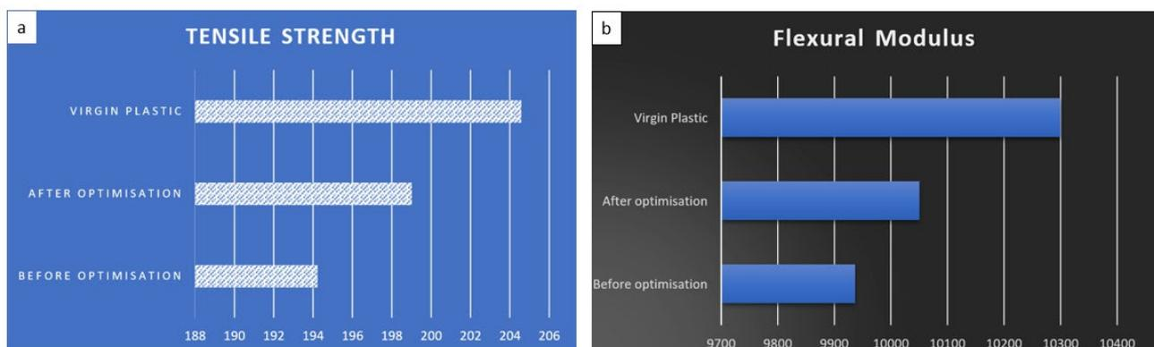
**Fig. 5.** (a) Tensile strength and (b) flexural modulus as comparisons before and after optimisation
