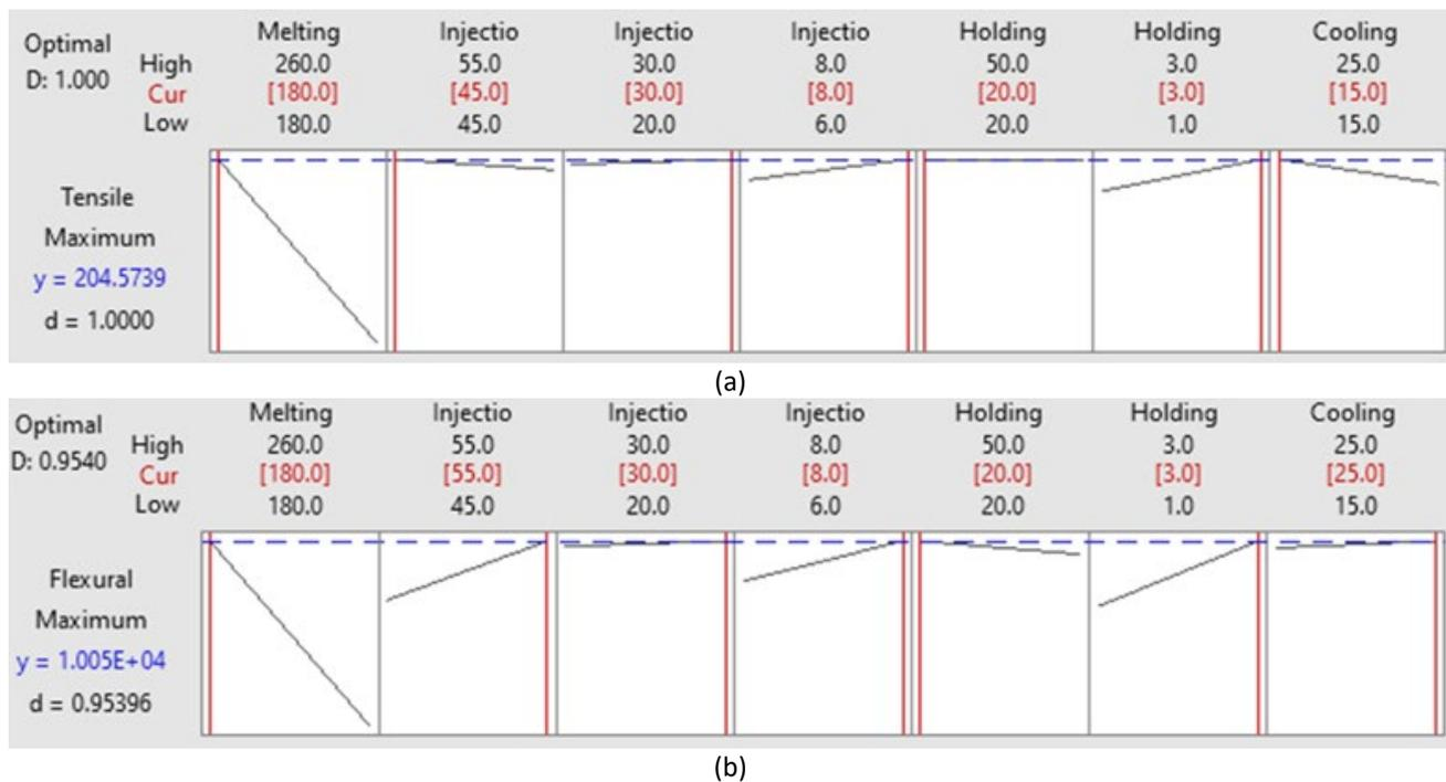
Fig. 4. (a) Tensile strength and (b) flexural modulus as responses for individual optimisation
