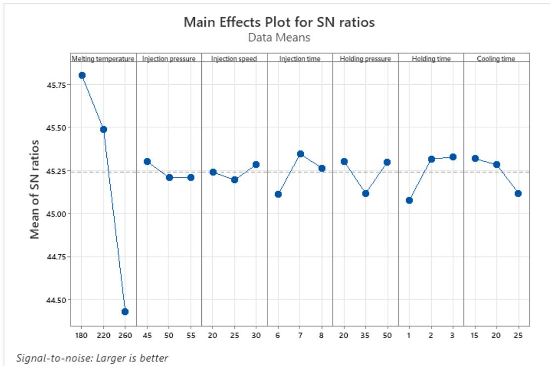
**Fig. 2.** Signal to noise ratio plot for compression strength
