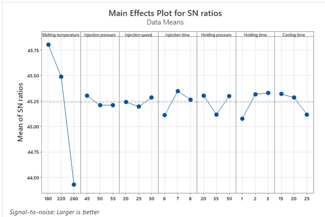
**Fig. 3.** Signal to noise ratio plot for flexural modulus
