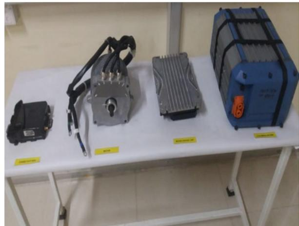
(b) Motor Controller, Motor, BMS module, Battery
