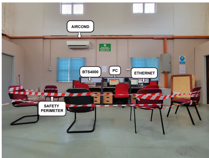
Fig. 3. Test bench for battery cell testing comprised of BTS400, PC, and internet access
