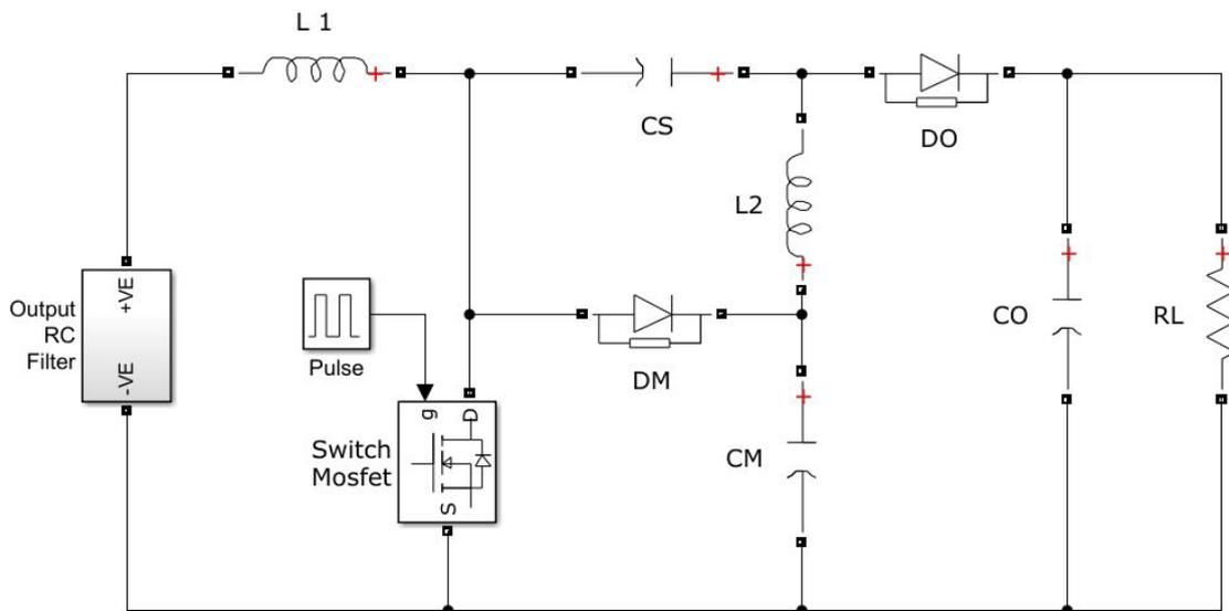
Fig. 3. Modified SEPIC Circuit
