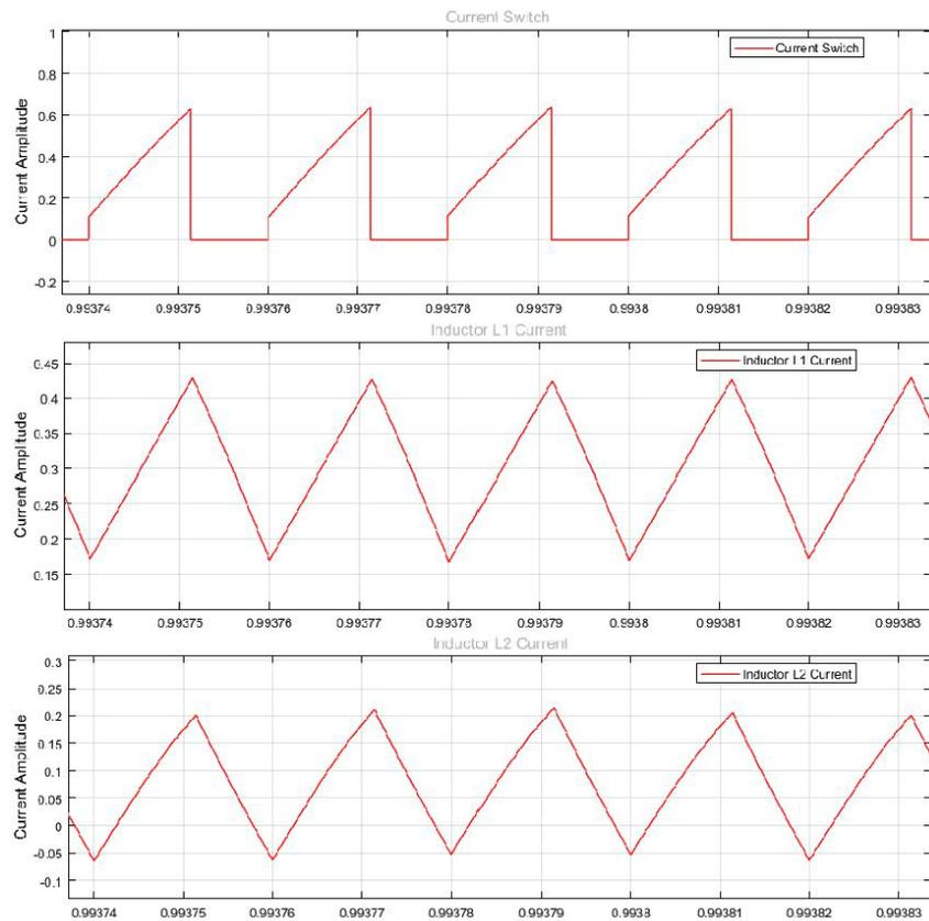
**Fig. 7.** Current Ripples of Modified SEPIC
