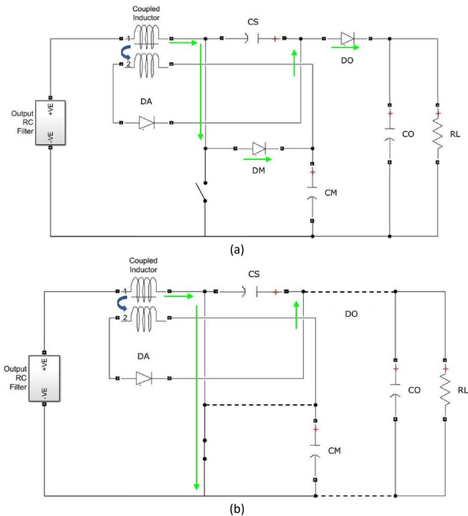
**Fig. 2.** Operation of Proposed Converter Design where (a) Off-state and (b) On-state
