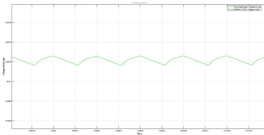
**Fig. 11.** Output Voltage Ripple of Proposed Design Converter
