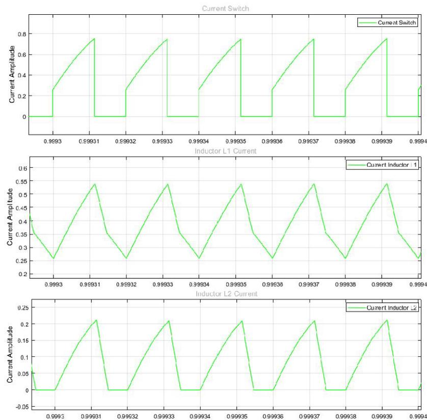
**Fig. 8.** Current Ripples of Proposed Design Converter
