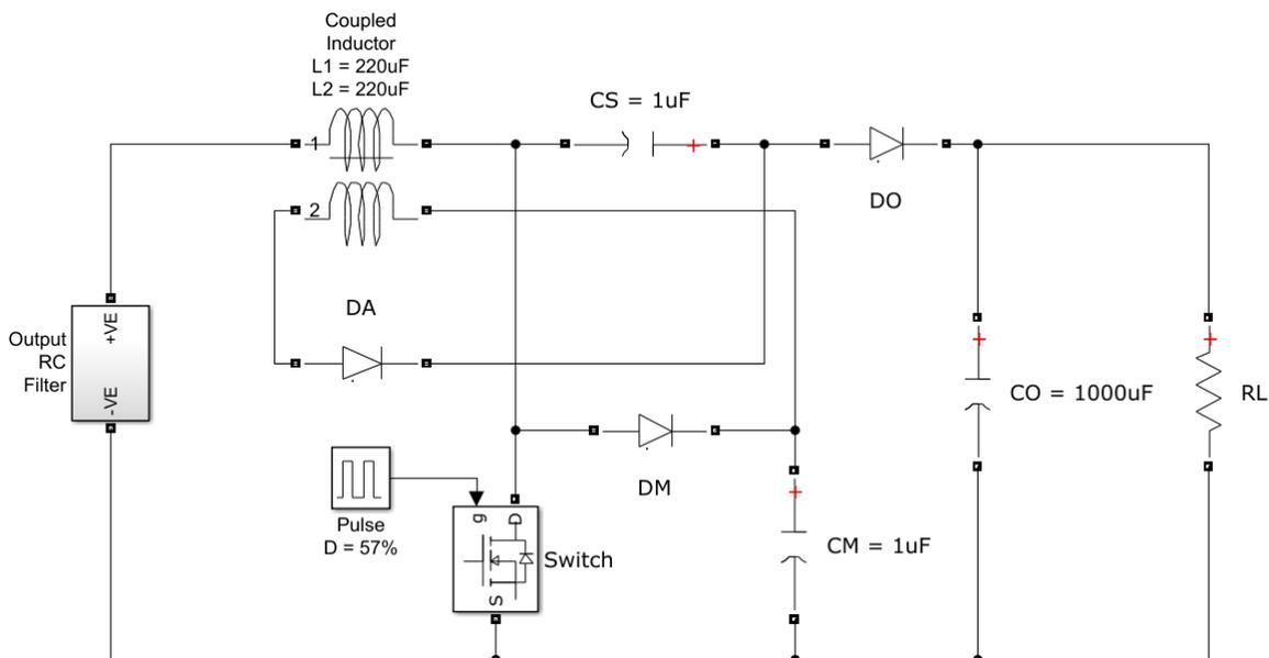
**Fig. 4.** Proposed Stabilizer Circuit
