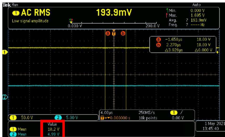
**Input Voltage = 4.99V    Output Voltage = 18.2V**
