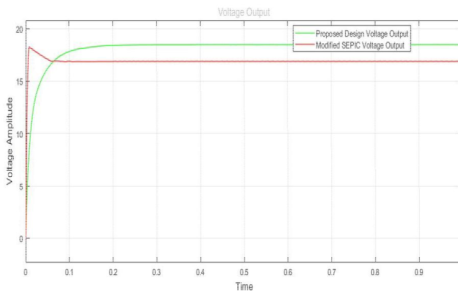
**Fig. 9.** Output Voltage of Proposed Converter vs Modified SEPIC Circuit
