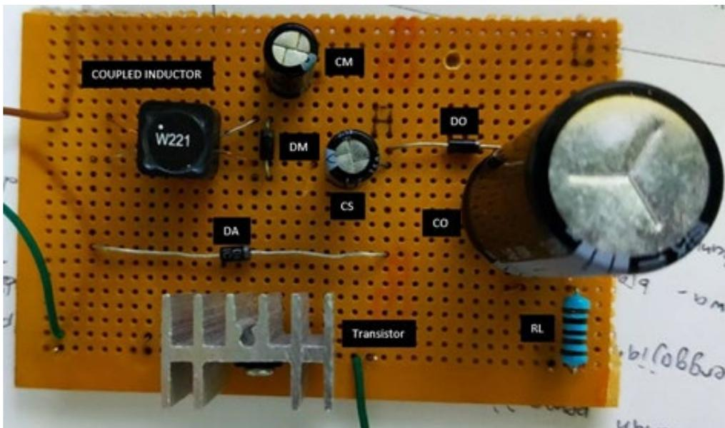
**Fig. 12.** Prototype of the Proposed Converter
