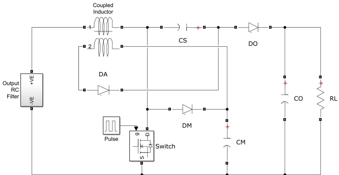
Fig. 1. Proposed Design Circuit
