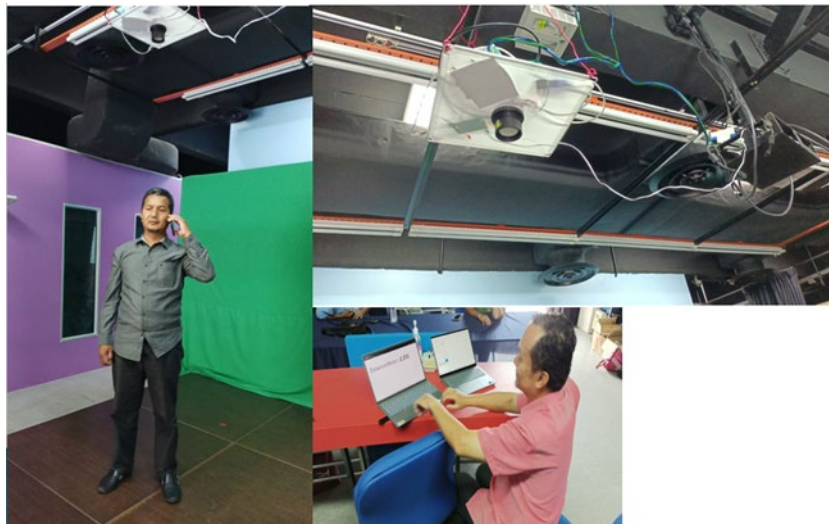
Fig. 5. System set up: (left) ultrasonic sensor, (right) RTU unit and (bottom) display unit
