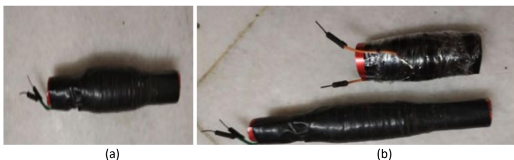
Fig. 8. (a) Wave generator for third attempt: 5.7 cm length (b) Wave generator for Fourth Attempt: 3 cm length
