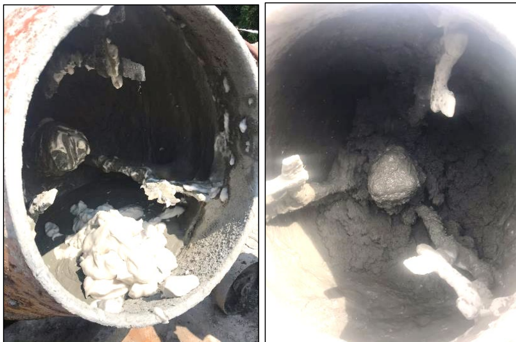
Fig. 3. LWFC mixing process
