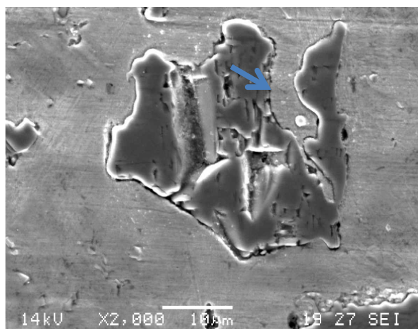
Fig. 4. A cracked particulate with an arrow showing matrix infiltration
