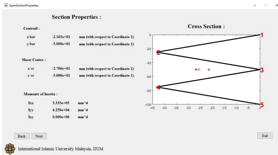
**Fig. 12.** Section properties window
