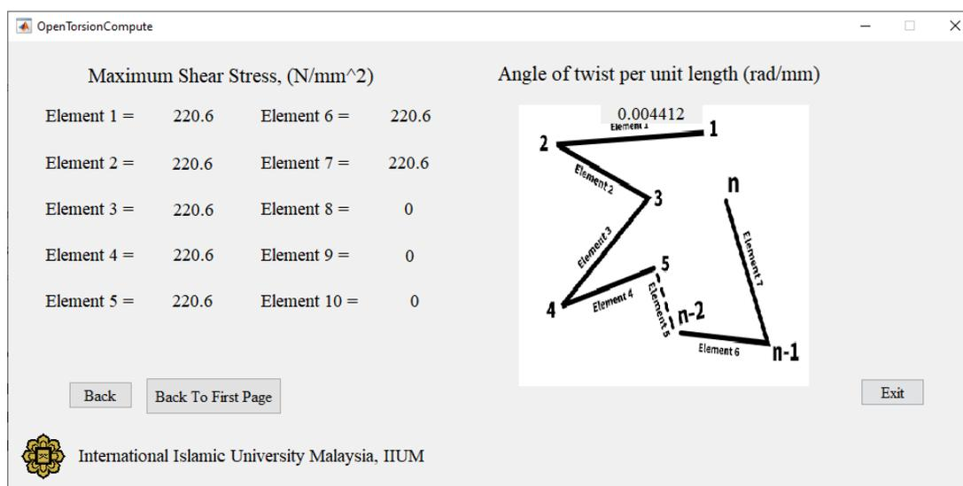
Fig. 25. Maximum shear stress and angle of twist per unit length result from the software
