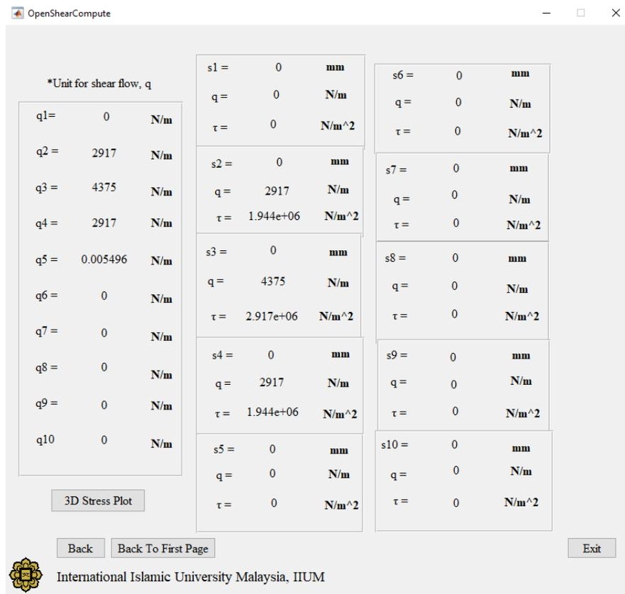
Fig. 22. Shear stress result from the software
