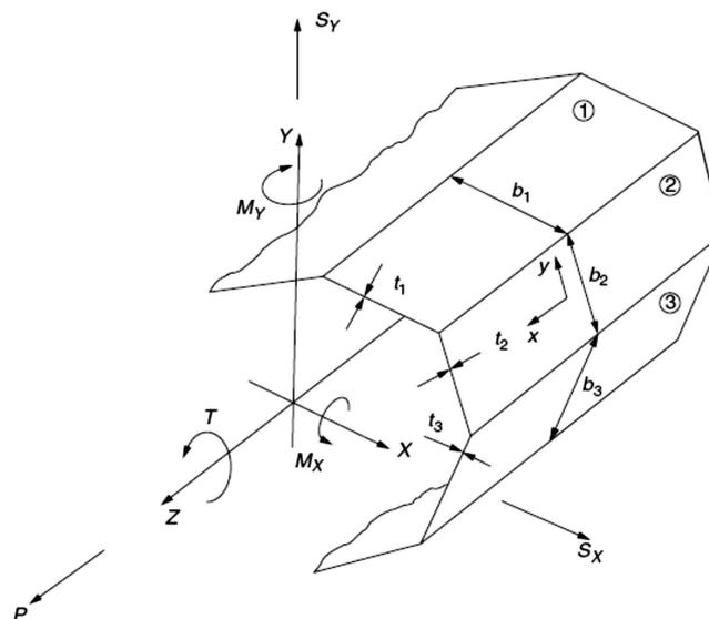
Fig. 3. Typical thin-walled section with loading
