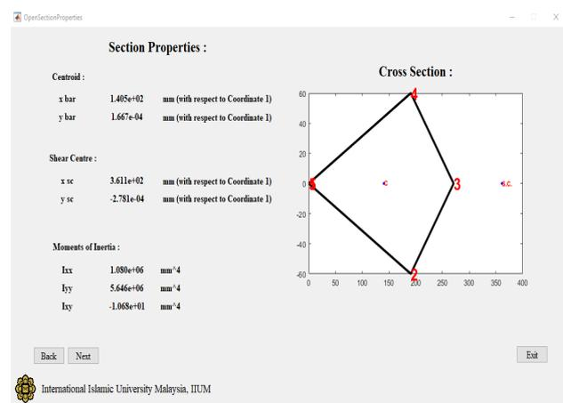
Fig. 20. Computed section properties
