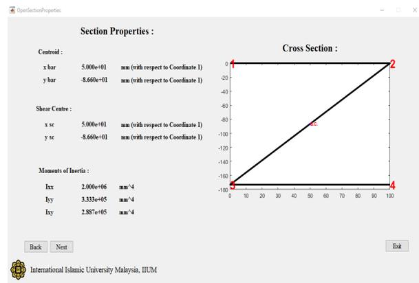
Fig. 15. Section Properties of the section
