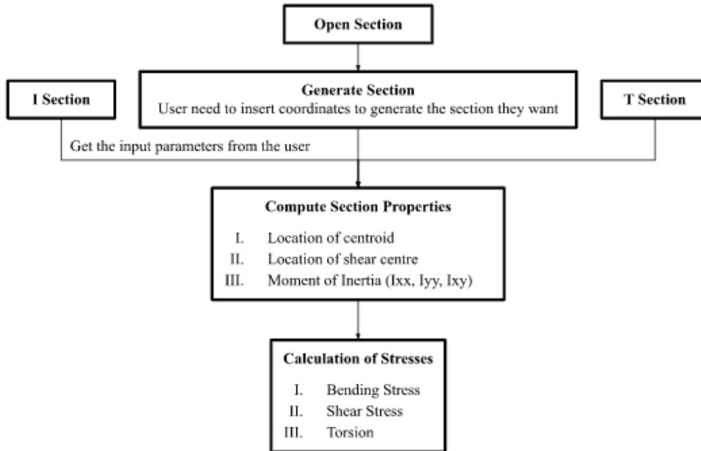
Fig. 4. Flow chart for the stress analysis
