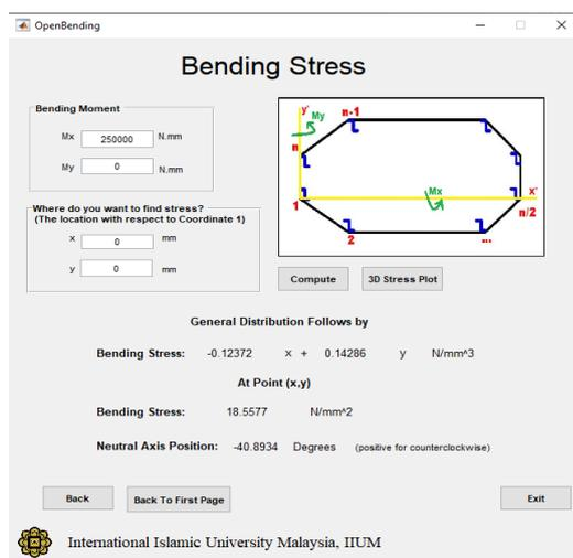
Fig. 16. Bending stress Input
