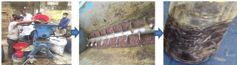
Extraction of cotton seed oil process
