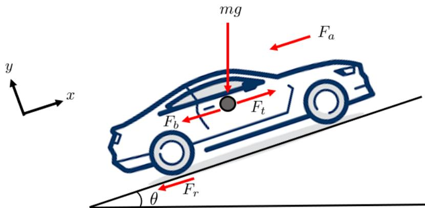
Fig. 2. Free body diagram for vehicle body [19]
