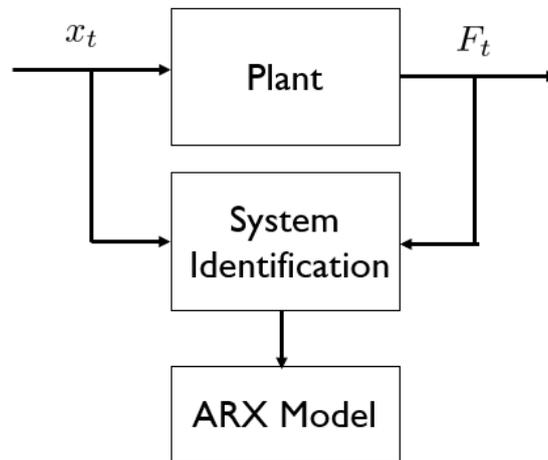
**Fig. 10.** System identification process for powertrain dynamics
