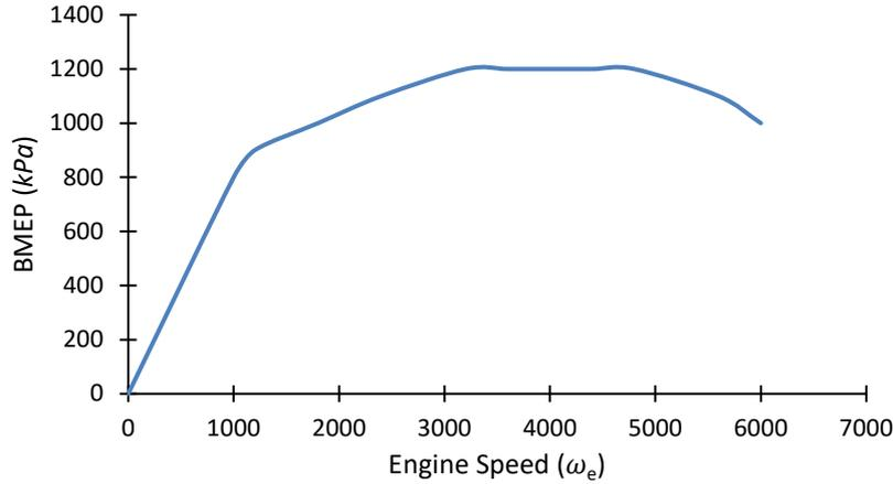
**Fig. 5.** Typical BMEP vs engine speed curve
