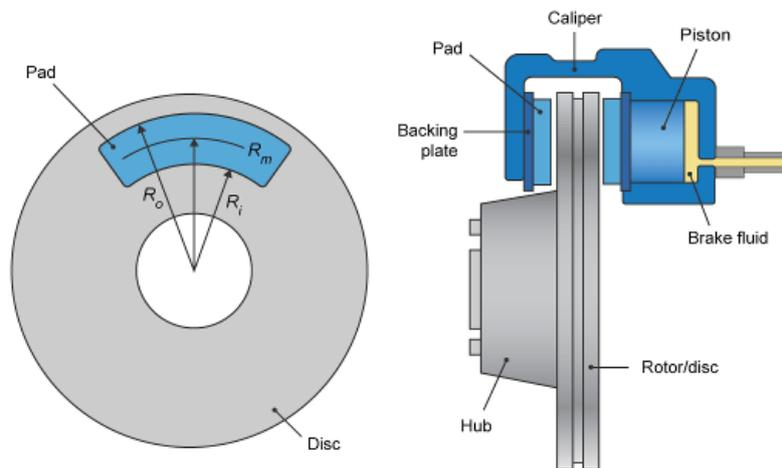
**Fig. 3.** Schematic of disk brake system [18]
