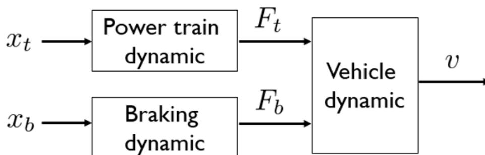
Fig. 1. Block diagram for longitudinal vehicle dynamic
