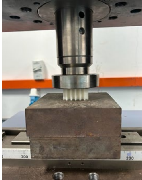
Fig. 3. Compression testing on 3D printed hollow and thin-walled structures
