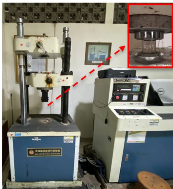
Fig. 4. The compressive strength test using UTM
