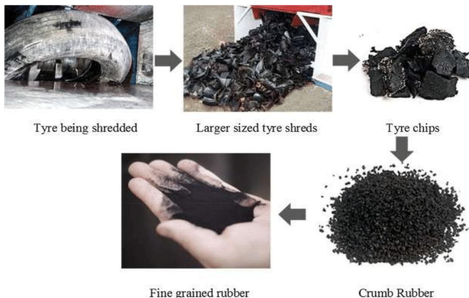
**Fig. 1.** Waste rubber production process [8]
