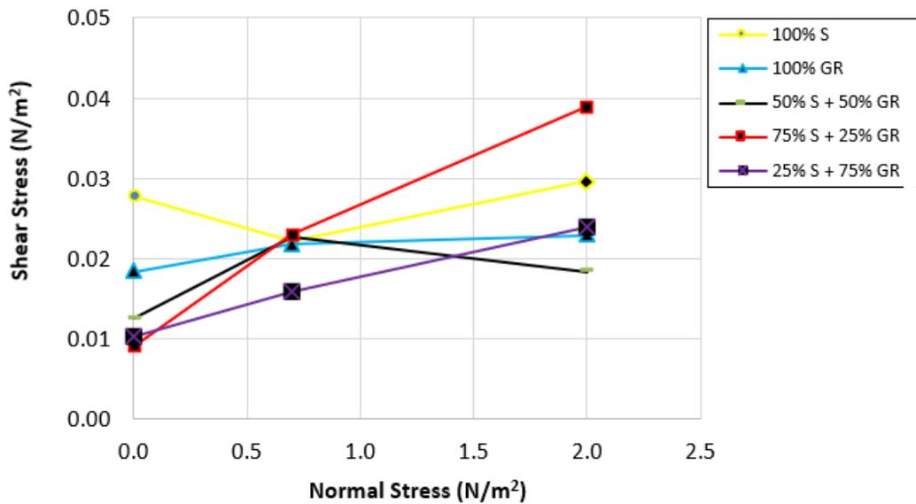
Fig. 7. Graph normal stress versus shear stress for GR (wet sample)
