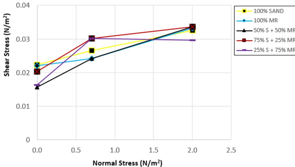
Fig. 9. Graph normal stress versus shear stress for MR (wet sample)
