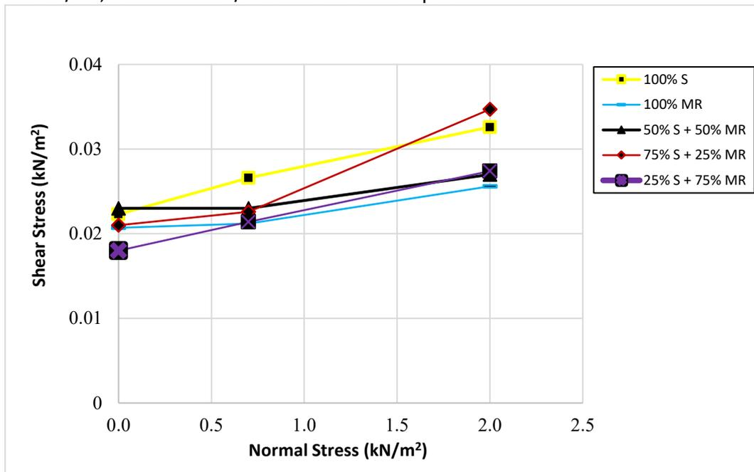
Fig. 8. Graph normal stress versus shear stress for MR (dry sample)
