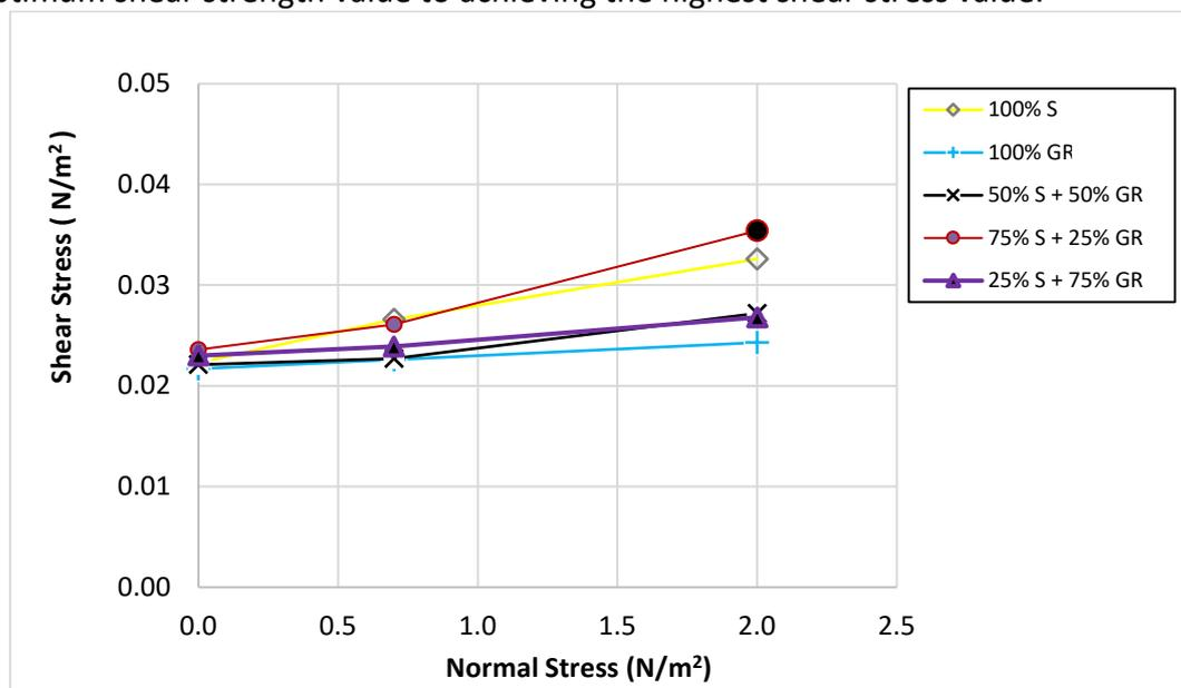
**Fig. 6.** Graph normal stress versus shear stress for GR (dry sample)
