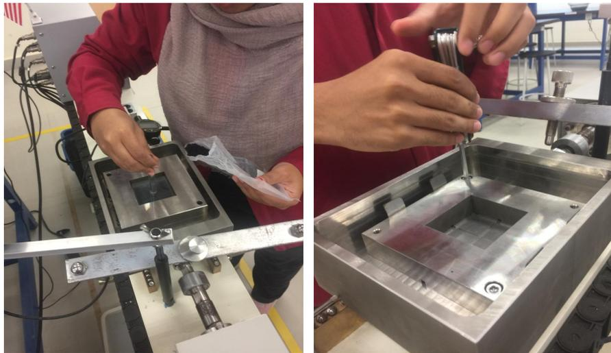
**Fig. 4.** Sample preparation into direct shear test machine
