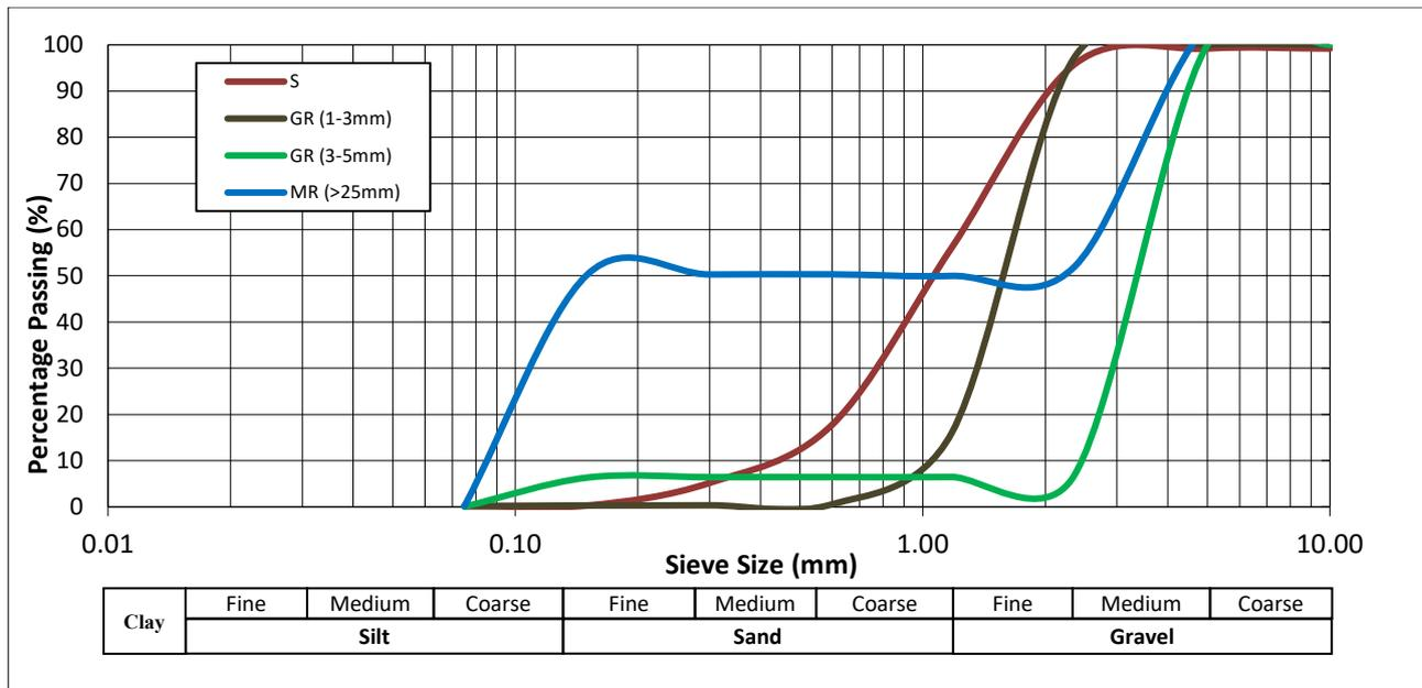
**Fig. 5.** Particle size distribution of the sand and waste rubber (GR and MR)
