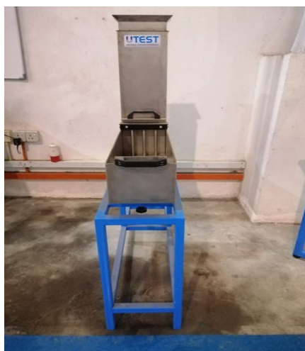
Fig. 4. Apparatus of the L-box test
