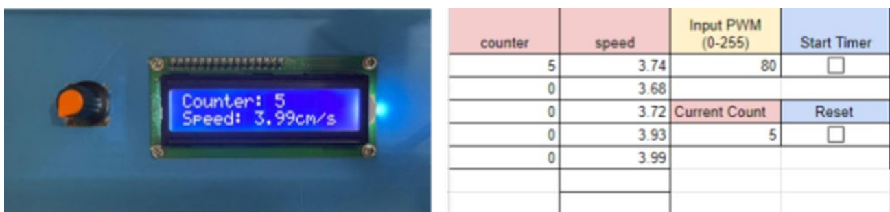
Fig. 7. Counter and speed parameters showing on LCD and Google Spreadsheet
