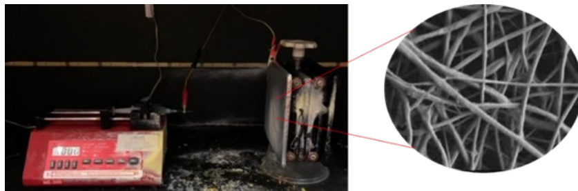
Fig. 1. A horizontal electrospinning setup was used in the experiment
