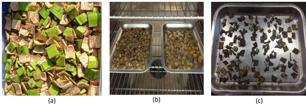
Fig. 1. Drying process (a) Banana peels (b) Sample in oven (c) Dried banana peels
