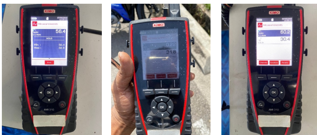
Fig. 7. Measurement of air temperature, velocity, and relative humidity inside and outside of the room using KIMO-AMI 310 Multifunction
