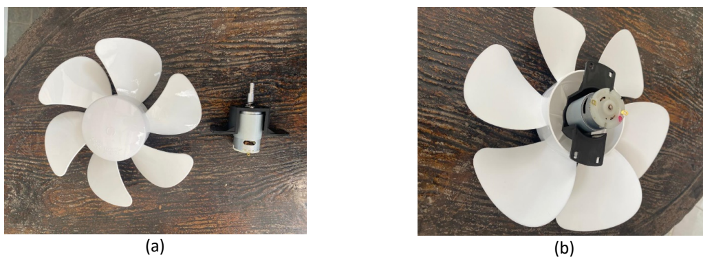
Fig. 2. DC exhaust fan (a) Front view (b) Rear view
