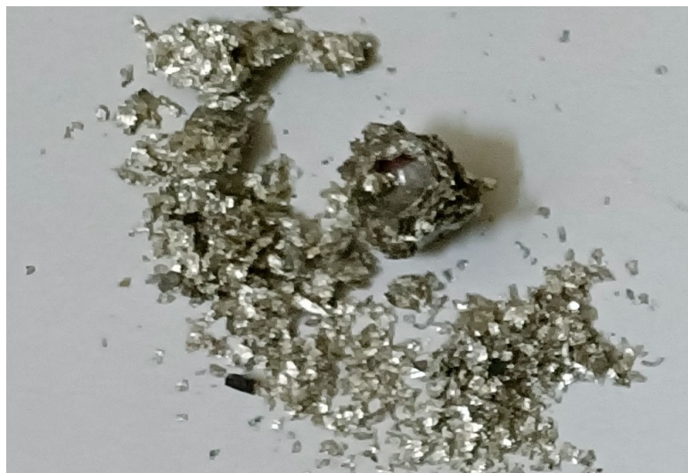
Fig. 11. Plug formation in recycled AA-6061 plates post impact
