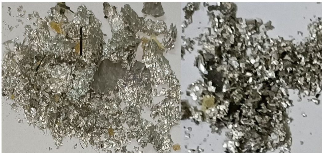
Fig. 12. Fragmentation in recycled AA-6061 plates post impact
