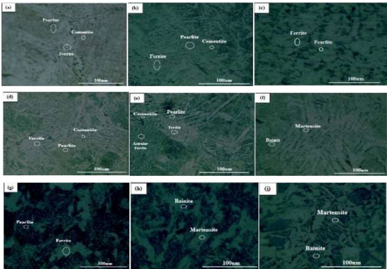
Fig. 3. Optical Microscope (OM) of CGHAZ with a 100x of magnification (a) Sample 1 (b) Sample 2 (c) Sample 3 (d) Sample 4 (e) Sample 5 (f) Sample 6 (g) Sample 7 (h) Sample 8 and (i) Sample 9
