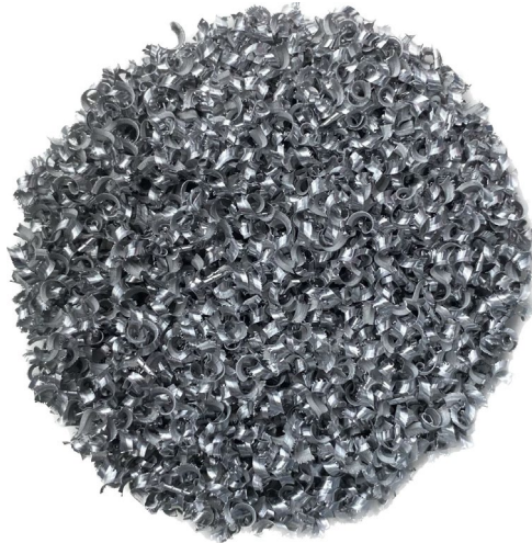
Fig. 1. Aluminium chips are produced from CNC machines
