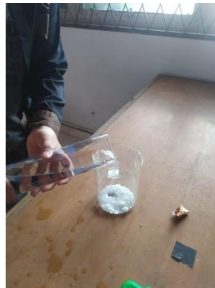
Fig. 2. Mixing NaOH with Aquadest
