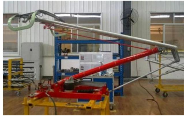
Fig. 2. Brecknell Willis TS-6034-type pantograph
