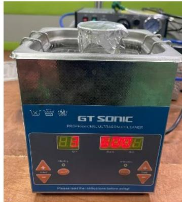
**Fig. 1.** The sonication process using an ultrasonic bath
