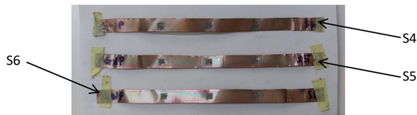
Fig. 5. Samples used for torsional test
